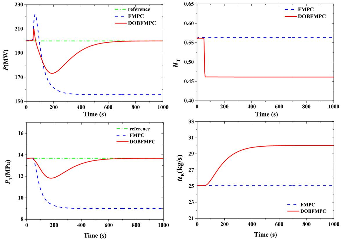
Fig. 10. Performance of the BTS with external disturbances: (left) outputs; (right) inputs.
