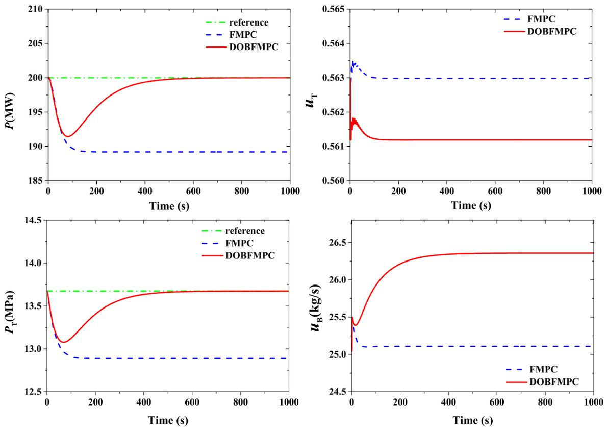
Fig. 12. Performance of the BTS with the model mismatch: (left) outputs; (right) inputs.
