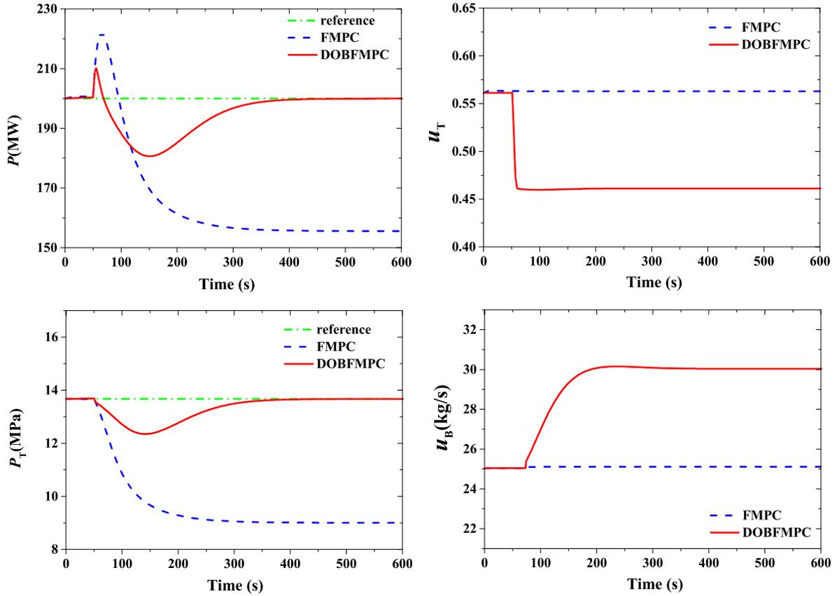
Fig. 13. Performance of the BTS with external disturbances in the mismatched case: (left) outputs; (right) inputs.
