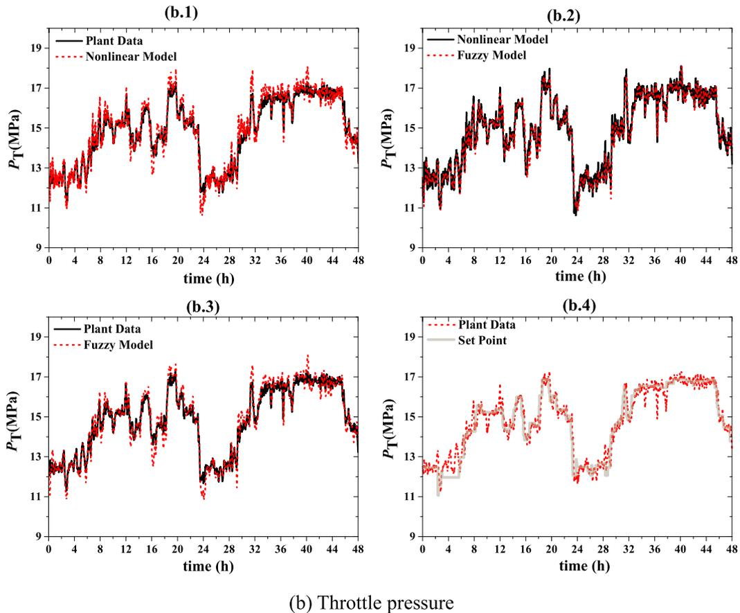
Fig. 4. The simulation results of the fuzzy model, the nonlinear model, plant data and the set points.
