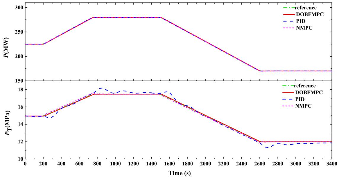
Fig. 5. Outputs of the BTS for a ramp-type load change: 225–280–170 MW.
