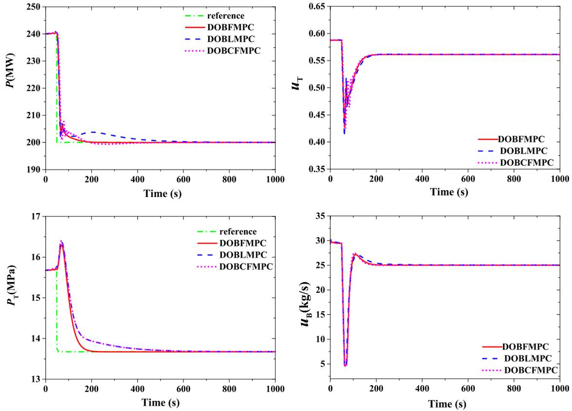
Fig. 9. Performances of the BTS for a step load change: 240-200 MW: (left) outputs; (right) inputs.
