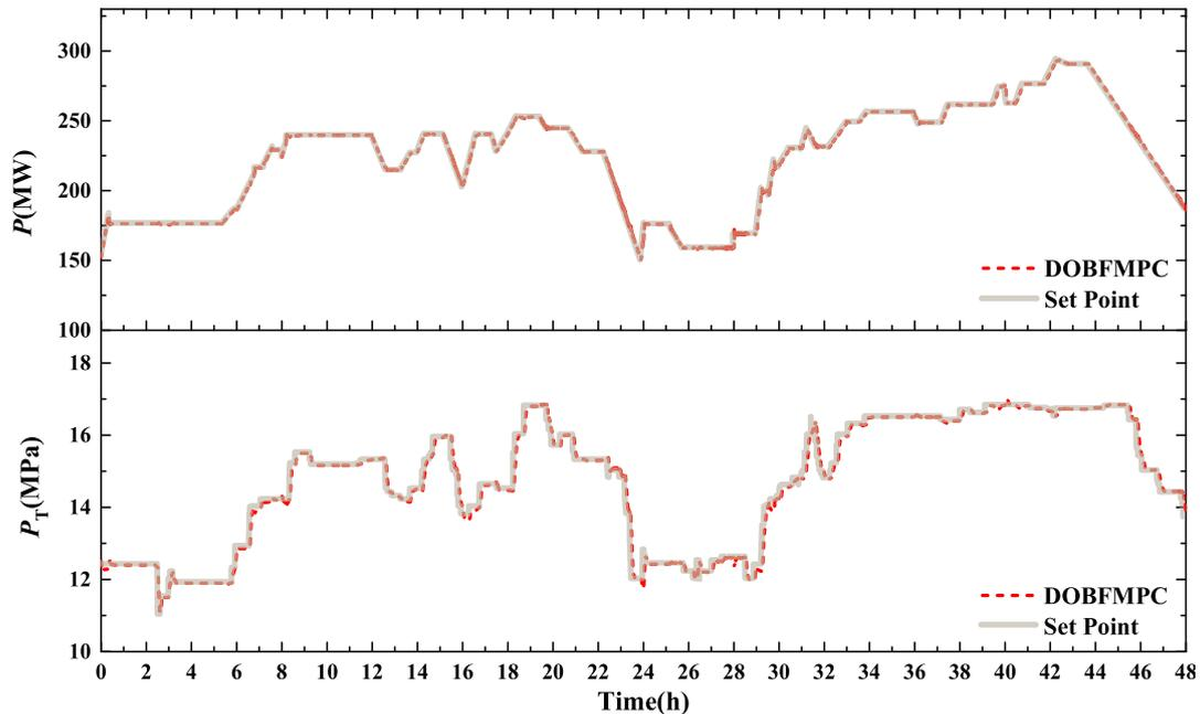
Fig. 8. Tracking performance of DOBFMPC for the plant set points of the BTS.
