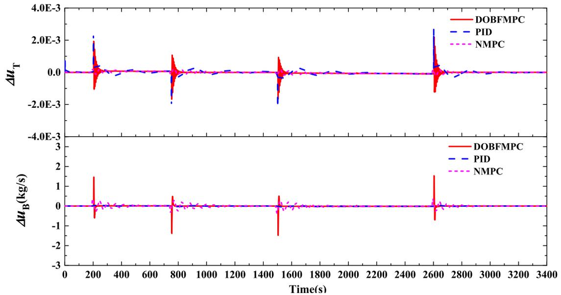
Fig. 7. Incremental inputs of the BTS for a ramp-type load change: 225–280–170 MW.
