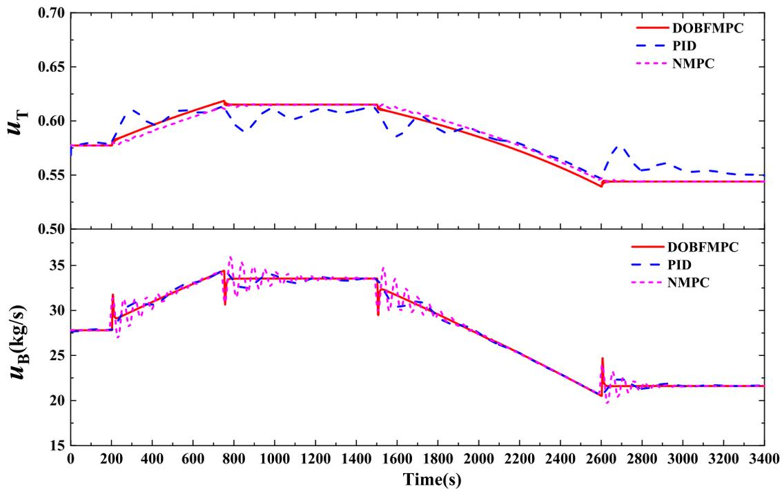
Fig. 6. Inputs of the BTS for a ramp-type load change: 225–280–170 MW.
