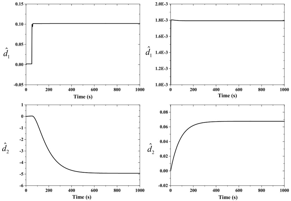
Fig. 11. Estimates of the disturbance term: (left) with external disturbances; (right) without external disturbances.
