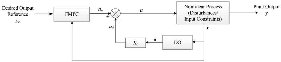
Fig. 1. The DOBFMPC scheme for the nonlinear process.
