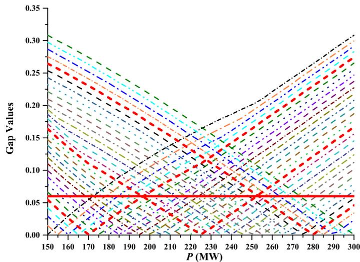
Fig. 2. The gap values between linearized models at equilibrium points.
