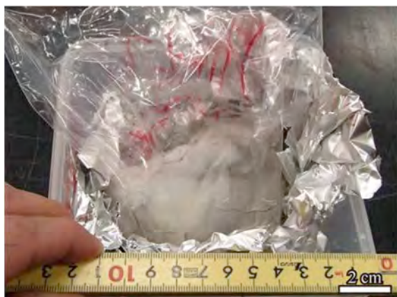
Fig. 3. Photograph of a sample undergoing ethanol substitution in preparation for the t -butyl alcohol freeze-drying method.
