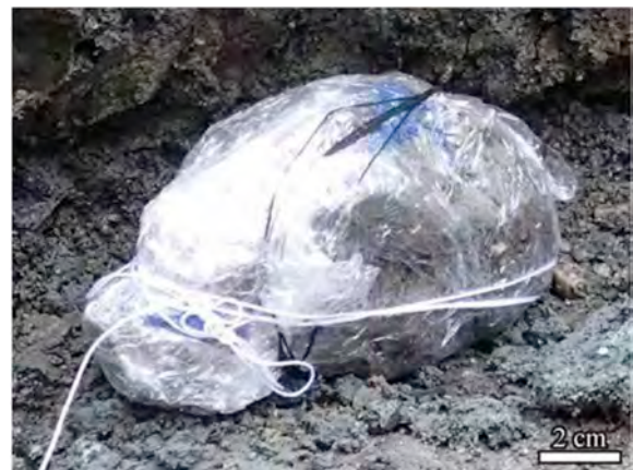
Fig. 2. Photograph of a bagged gouge sample in the field.
