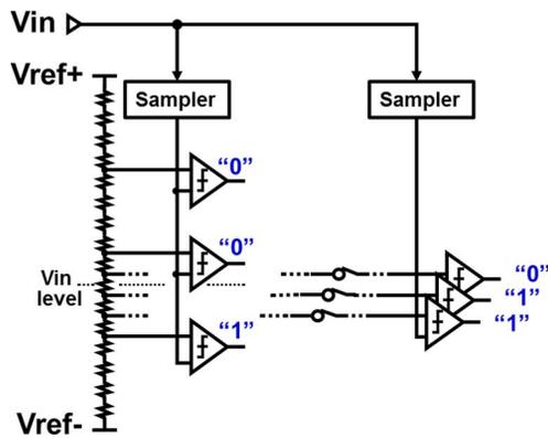
Fig. 1. Block diagram of operation of a 2-bit + 2-bit subranging ADC.
