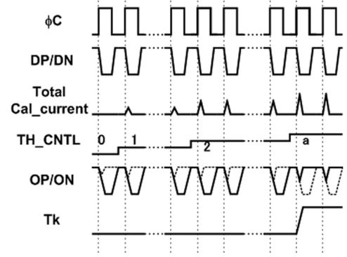
Fig. 10. Timing diagram for controlling the comparator's threshold level.
