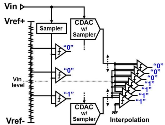
Fig. 2. Block diagram of the conventional circuit with the interpolation scheme.
