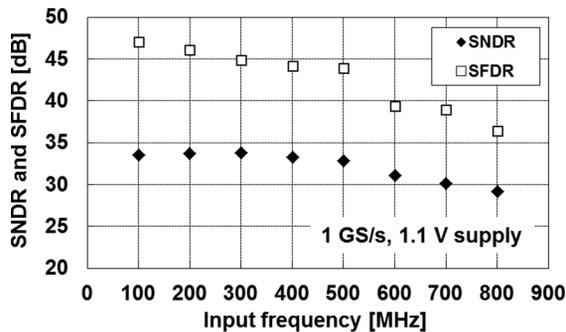
Fig. 15. SNDR and SFDR vs. input frequency.
