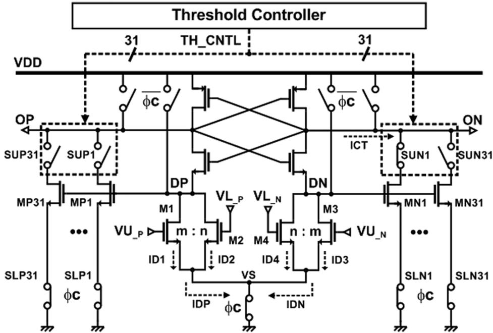
Fig. 8. Schematic diagram of comparator with circuits for controlling the threshold level.
