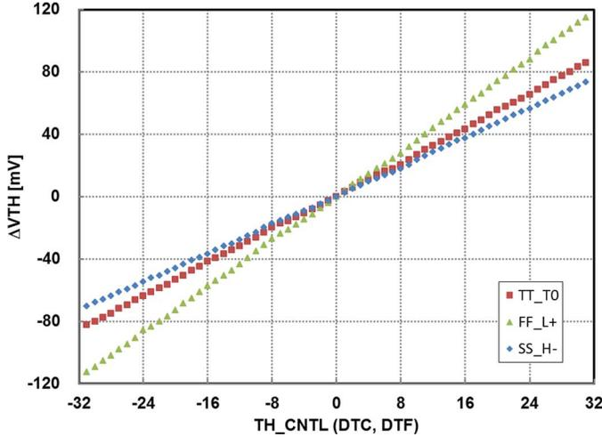
Fig. 9. Simulated controllable range of the comparator's threshold level vs. control code. TT\_T0: Typically,  $T = 25^\circ\text{C}$ ,  $V_{DD} = 1.2\text{ V}$ , FF\_L+: Fast,  $T = -40^\circ\text{C}$ ,  $V_{DD} = 1.3\text{ V}$ , SS\_H-: Slow,  $T = 125^\circ\text{C}$ ,  $V_{DD} = 1.1\text{ V}$ .
