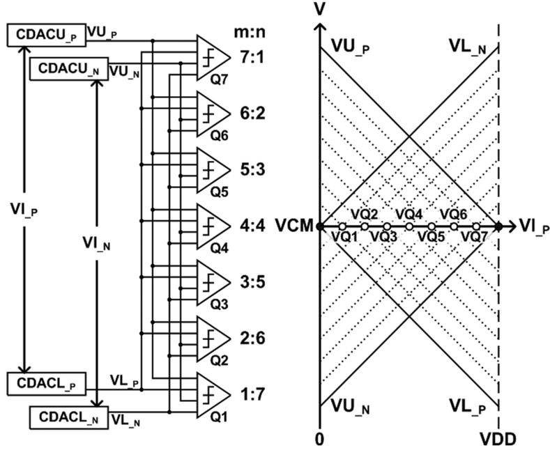
Fig. 7. Interpolation of signals with the proposed circuit.
