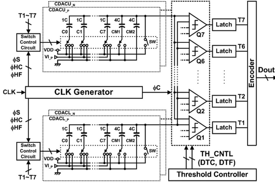
Fig. 3. Block diagram of the proposed ADC.
