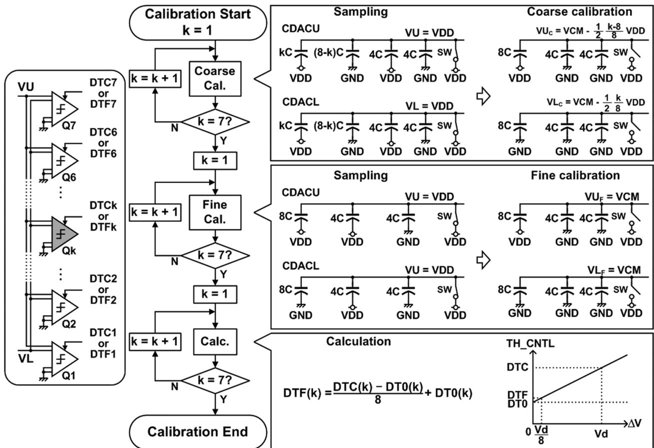
Fig. 11. Flow chart for the foreground calibration.
