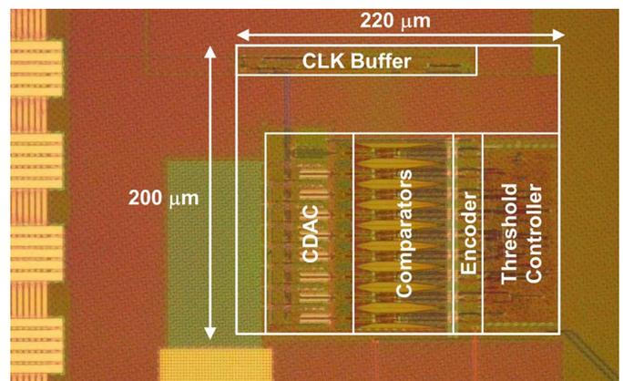
Fig. 12. Chip micrograph.
