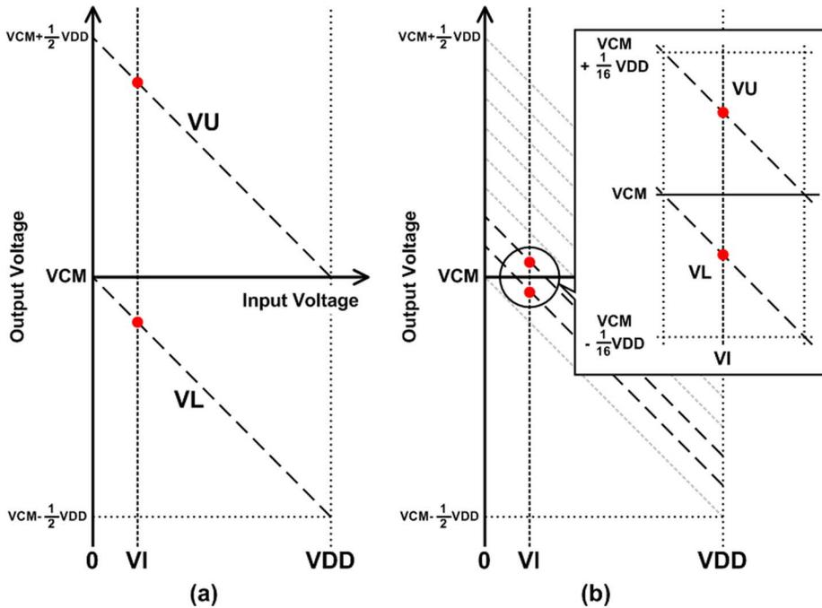
Fig. 6. Conceptual diagram of CDAC output (a) for coarse decision and (b) for fine decision.
