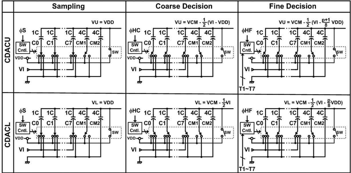
Fig. 5. Operational diagram of CDACs.
