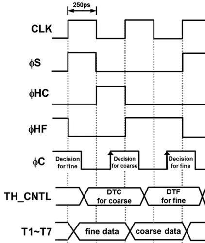
Fig. 4. Timing diagram of the proposed ADC.
