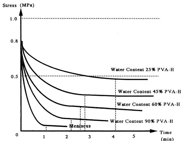
Fig. 4. Comparison of the stress–relaxation curves of PVA-H and meniscus specimens.
