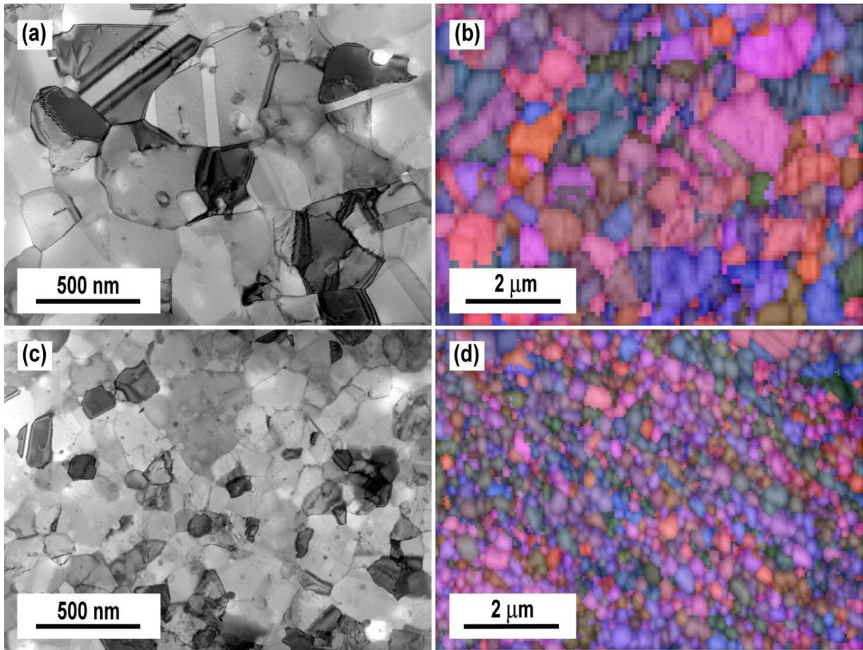
Fig. 2 Grain structure of SPSed HEA (up) and ODS HEA (down) visualised by STEM (left) and EBSD SEM (right).
