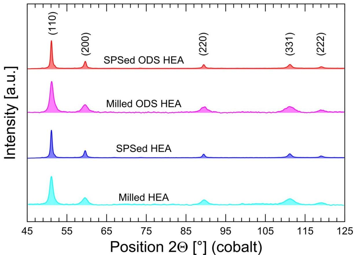
Fig. 1 XRD patterns of HEA and ODS HEA alloyed powders and SPSed compacts.
