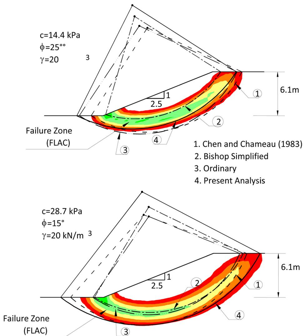
**Fig. 10.** Comparison for failure surfaces obtained from different methods
