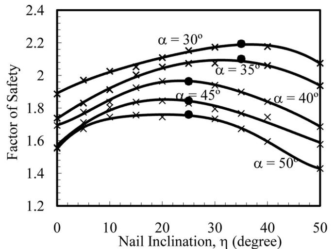
**Fig. 12.** Influence of nail inclination and slope angle on FS values of soil-nailed slopes
