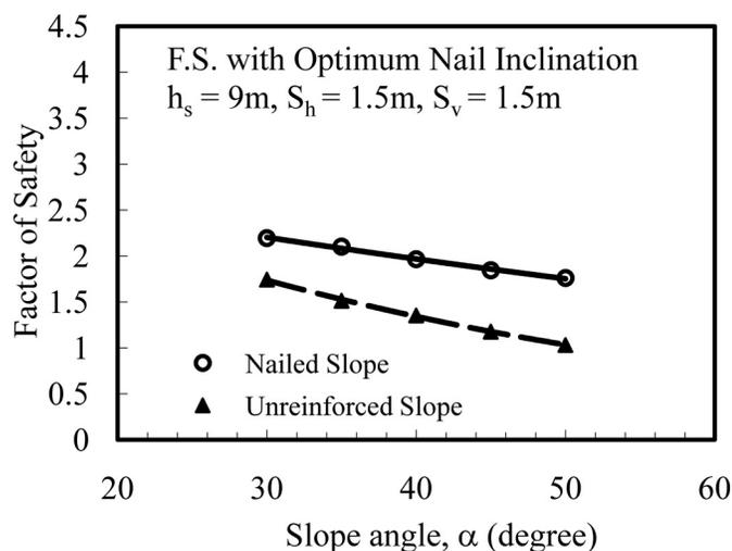
**Fig. 13.** Influence of slope angle on increase in FS values of soil-nailed slopes
