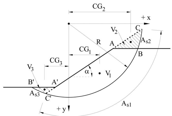
Fig. 5. Scheme for computation of the surface area: discretization of failure block
