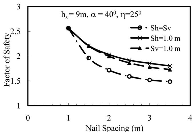
**Fig. 14.** Effect of nail spacing on FS values of soil-nailed slopes
