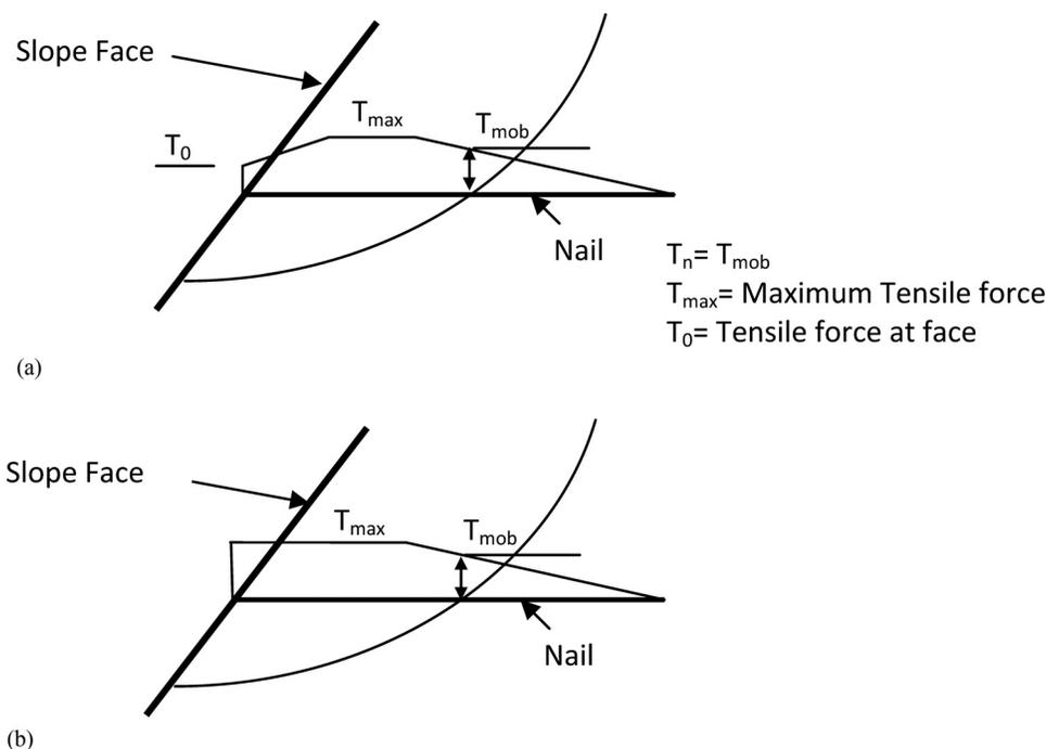
Fig. 8. Tensile force distribution in nail: (a) FHWA guidelines; (b) considered in present analysis
