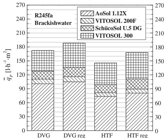
**Fig. 9.** Influence of solar cycle configuration over the unit volumetric flow rate of desalted water. Solar ORC with R245fa as working fluid and brackish water at  $20\ ^\circ C$  as feed water of RO unit.
