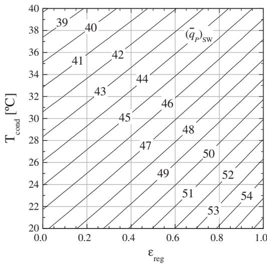
**Fig. 6.** Influence of condensation temperature and regeneration effectiveness over the unit volumetric flow rate of desalted water [ $l\ h^{-1}\ m^{-2}$ ]. Solar HTF ORC with VITOSOL 300, R245fa as working fluid, and seawater at  $20\ ^\circ C$  as feedwater of RO unit.
