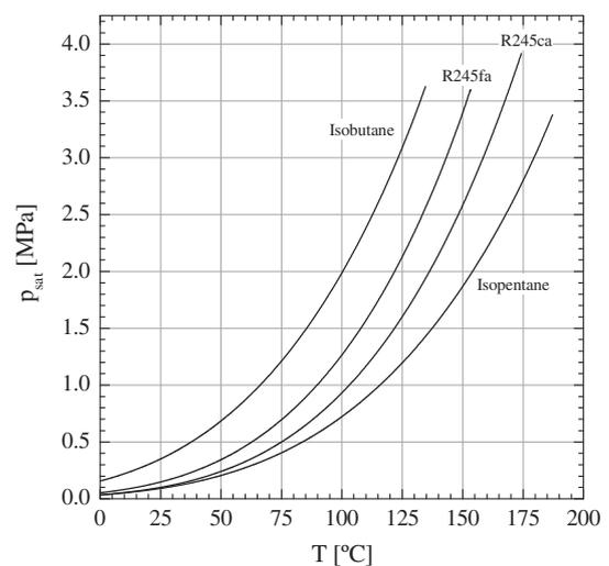
**Fig. 3.** Saturation pressure of R245ca, R245fa, isobutane and isopentane.
