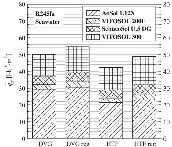
**Fig. 8.** Influence of solar cycle configuration over the unit volumetric flow rate of desalted water. Solar ORC with R245fa as working fluid and seawater at  $20\ ^\circ C$  as feed water of RO unit.
