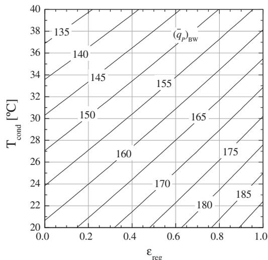
**Fig. 7.** Influence of condensation temperature and regeneration effectiveness over the unit volumetric flow rate of desalted water [ $l\ h^{-1}\ m^{-2}$ ]. Solar HTF ORC with VITOSOL 300, R245fa as working fluid, and brackish water at  $20\ ^\circ C$  as feedwater of RO unit.
