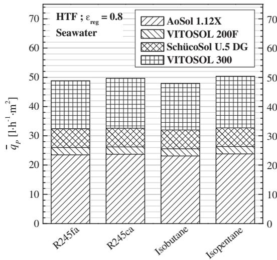
Fig. 4. Unit volumetric flow rate of desalted water as a function of working fluid and solar collector model for the seawater RO solar desalination system. Power cycle: HTF solar regenerative organic Rankine cycle.  $T_{cond} = 30 \text{ }^\circ\text{C}$ ,  $G = 1000 \text{ W/m}^2$ .
