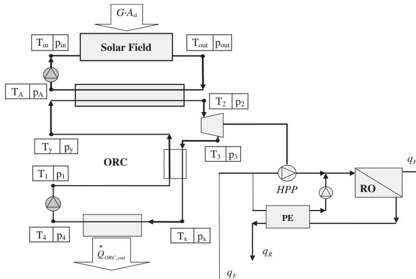
Fig. 1. Basic layout of the low-temperature solar thermal driven reverse osmosis desalination system in a heat transfer fluid configuration of the solar cycle.
