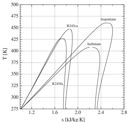
**Fig. 2.** Temperature-entropy diagrams of R245ca, R245fa, isobutane and isopentane.
