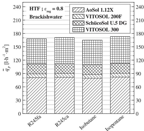
Fig. 5. Unit volumetric flow rate of desalted water as a function of working fluid and solar collector model for the brackish water RO solar desalination system. Power cycle: HTF solar regenerative organic Rankine cycle.  $T_{cond} = 30 \text{ }^\circ\text{C}$ ,  $G = 1000 \text{ W/m}^2$ .
