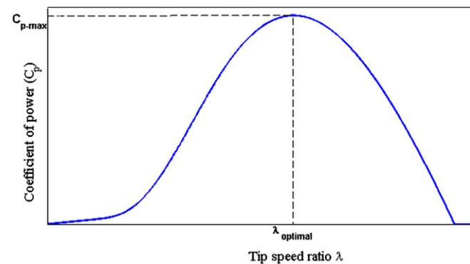
Fig. 3. The characteristic of the power coefficient as a function of tip speed ratio.
