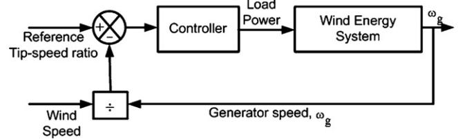
Fig. 5. The block diagram of the tip speed ratio control [1].
