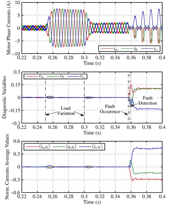
Fig. 5. Simulation results concerning the time-domain waveforms of the motor phase currents, the diagnostic variables, and the normalized currents average values, for a double power switch open-circuit fault in IGBTs T1 and T3.
