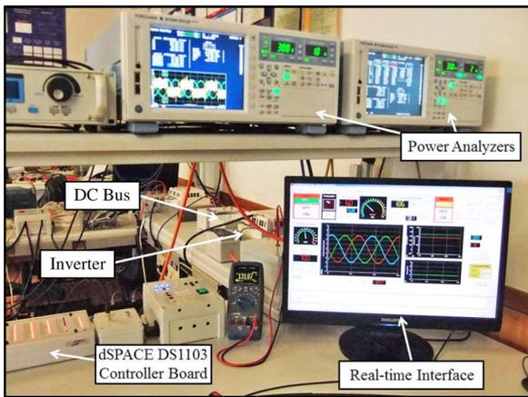
Fig. 7. General view of the power and control stages.
