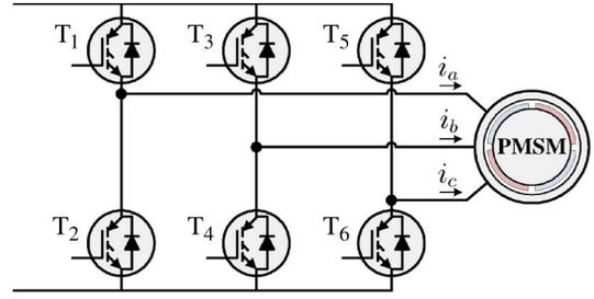
Fig. 2. Diagram of a typical VSI feeding a PMSM.
