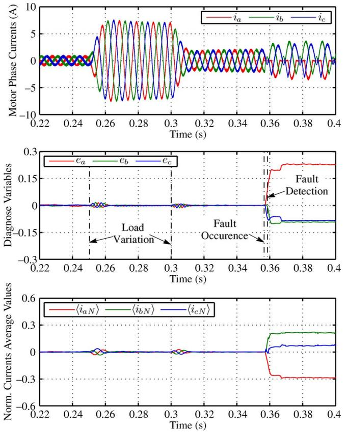
Fig. 3. Simulation results concerning the time-domain waveforms of the motor phase currents, the diagnostic variables, and the normalized currents average values, for a single power switch open-circuit fault in IGBT T1.
