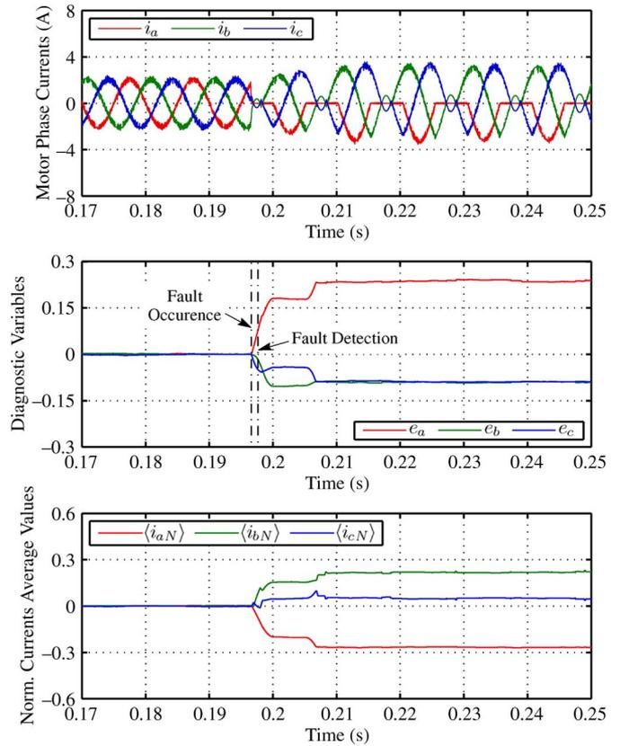
Fig. 9. Experimental results concerning the time-domain waveforms of the motor phase currents, the diagnostic variables, and the normalized currents' average values, for a single power switch open-circuit fault in IGBT T1.
