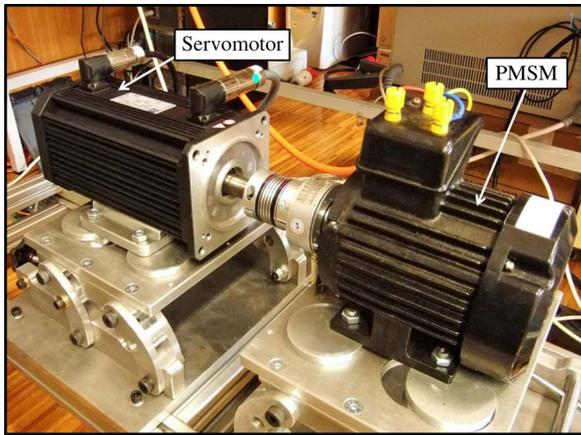
Fig. 6. Detail of the PMSM coupled to the servo machine.
