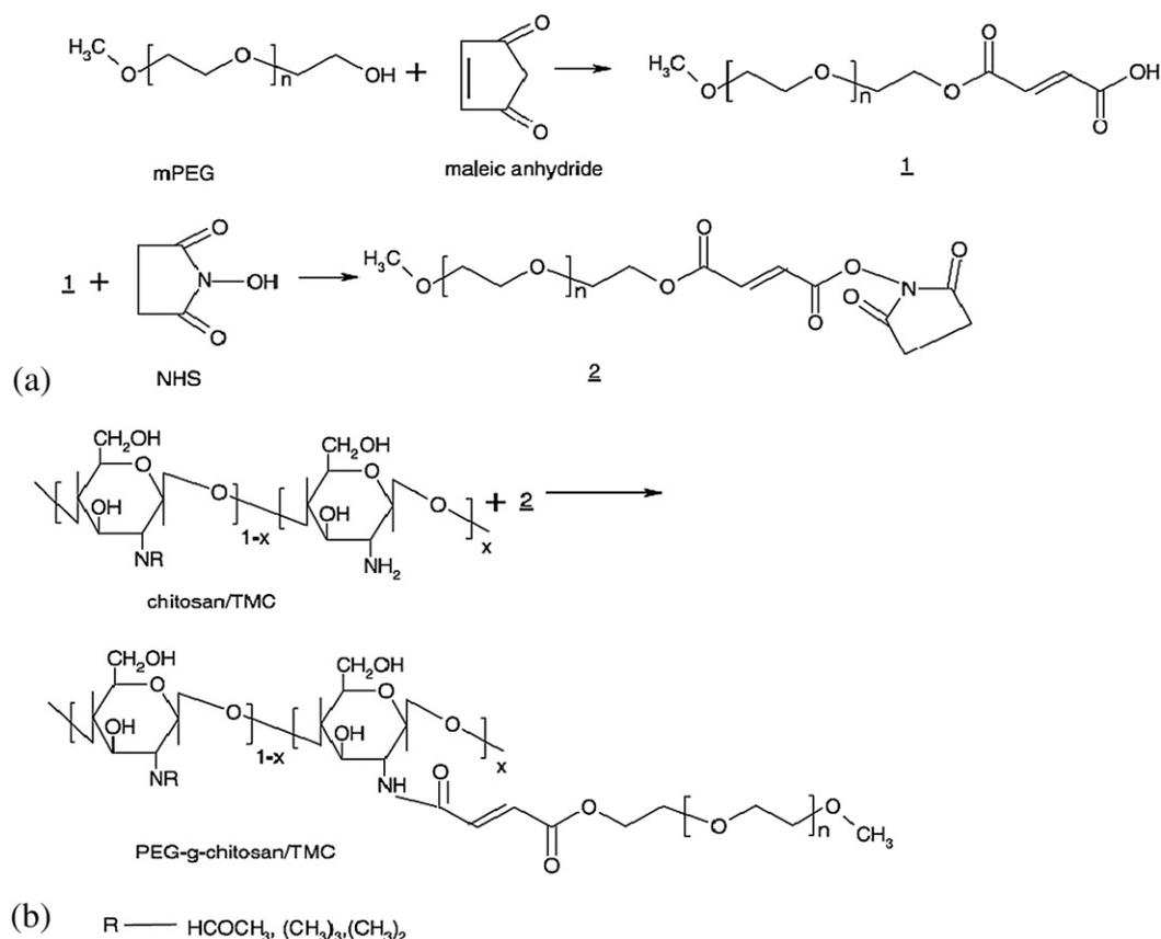
Fig. 4. Synthetic route of PEGylated chitosan derivatives (Mao et al., 2005).
