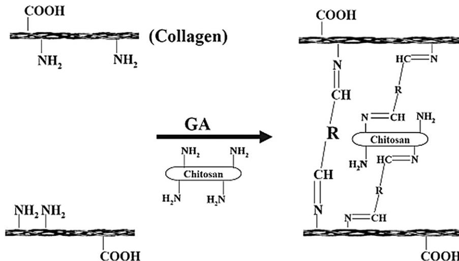
Fig. 7. Schematic presentation of collagen cross-linked with glutaraldehyde in the presence of chitosan (Schul et al., 2000).
