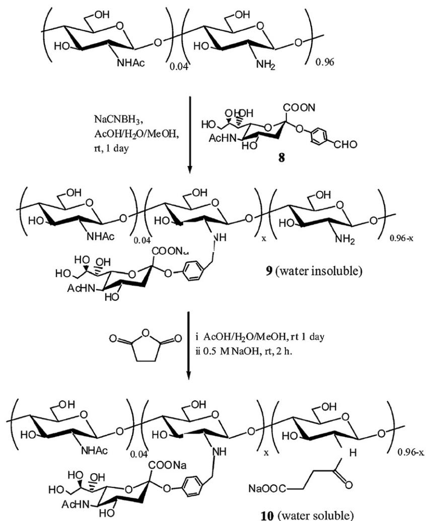
Fig. 2. Synthesis of sialic acid-chitosan and its *N*-succinylation (Gamian et al., 1991).
