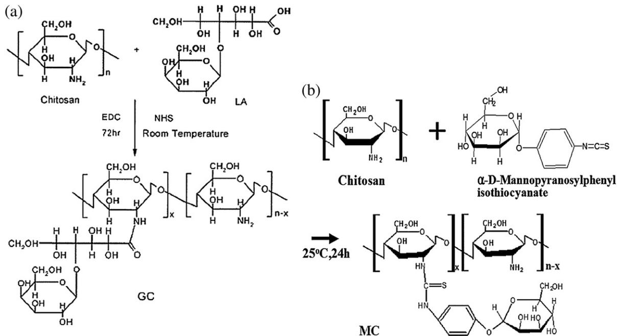
Fig. 1. Synthesis scheme of galactosylated chitosan (Park et al., 2003) (a) and mannosylated chitosan (Kim et al., 2006b) (b).
