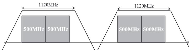
Fig. 4. The number of duplex filters to cover bandwidth to meet the needed data rate in 28 GHz band.
