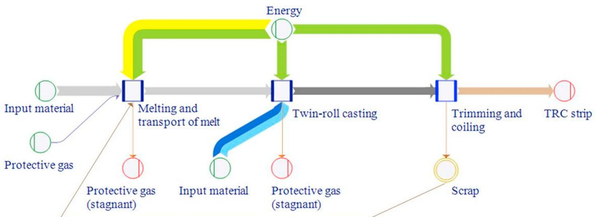
Fig. 3. Sankey diagram of stable twin-roll casting phase.
