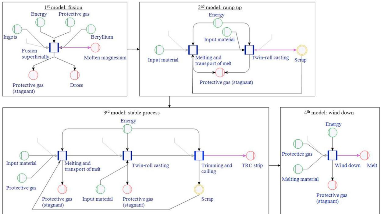
Fig. 2. Material flow models for twin-roll casting of AZ31 magnesium strips.
