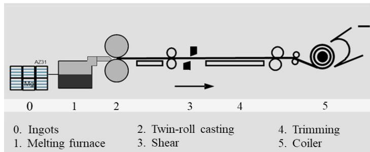
Fig. 1. Schematic illustration of twin-roll casting process based on [9].
