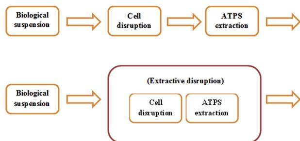
FIG. 2. Simplified representation of two flow diagrams in downstream processing for comparison. The upper flow diagram represents the conventional discrete process in which the cell disruption process is followed by an ATPS-based extraction process. On the other hand, the integrated process (extractive disruption) wherein cell disruption and ATPS were integrated into one step is presented in the lower diagram.
