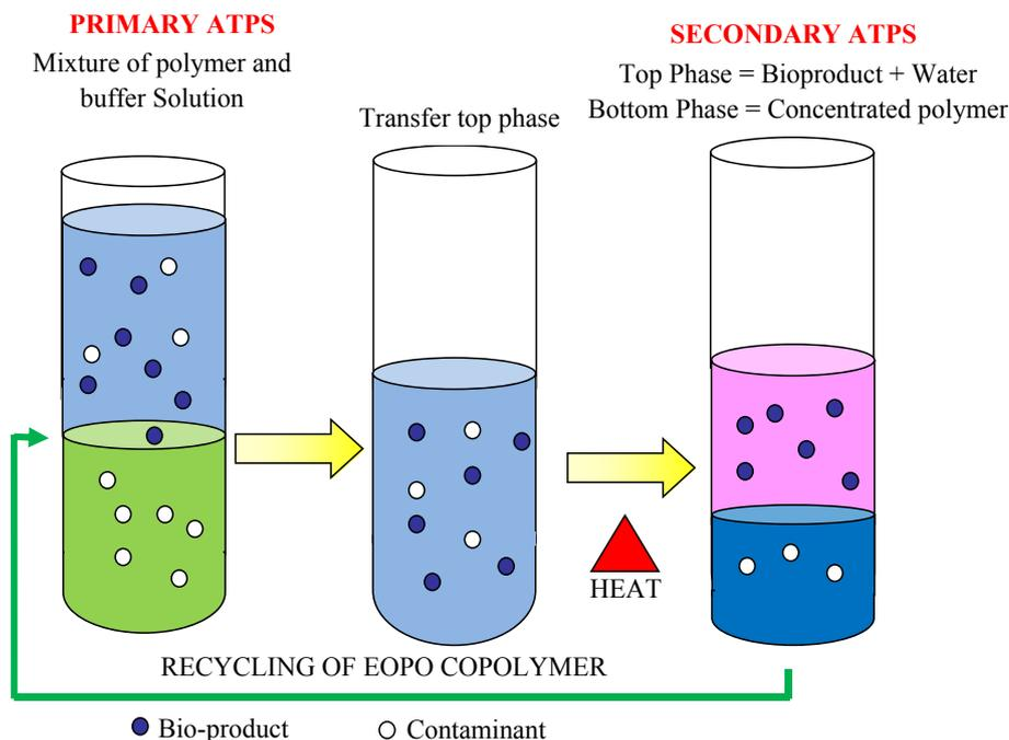
FIG. 3. This is a schematic diagram of the recycling ATPS using thermos-separating polymer. In the primary ATPS, the top phase contains desired bio-products will be separated to another test tube. Then it will be heated above critical solution temperature and form two phases. This will be called secondary ATPS. The top phase consists only water and pure bio-products while the bottom phase consists of concentrated polymer which can be re-used for a new ATPS. Modified from Show et al. (36).
