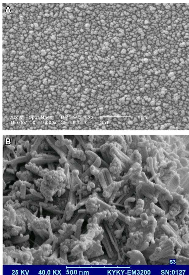
**Fig. 1** SEM of synthesized SnO<sub>2</sub> at **a** 0.02 M, **b** 0.03 M concentration of tin chloride
