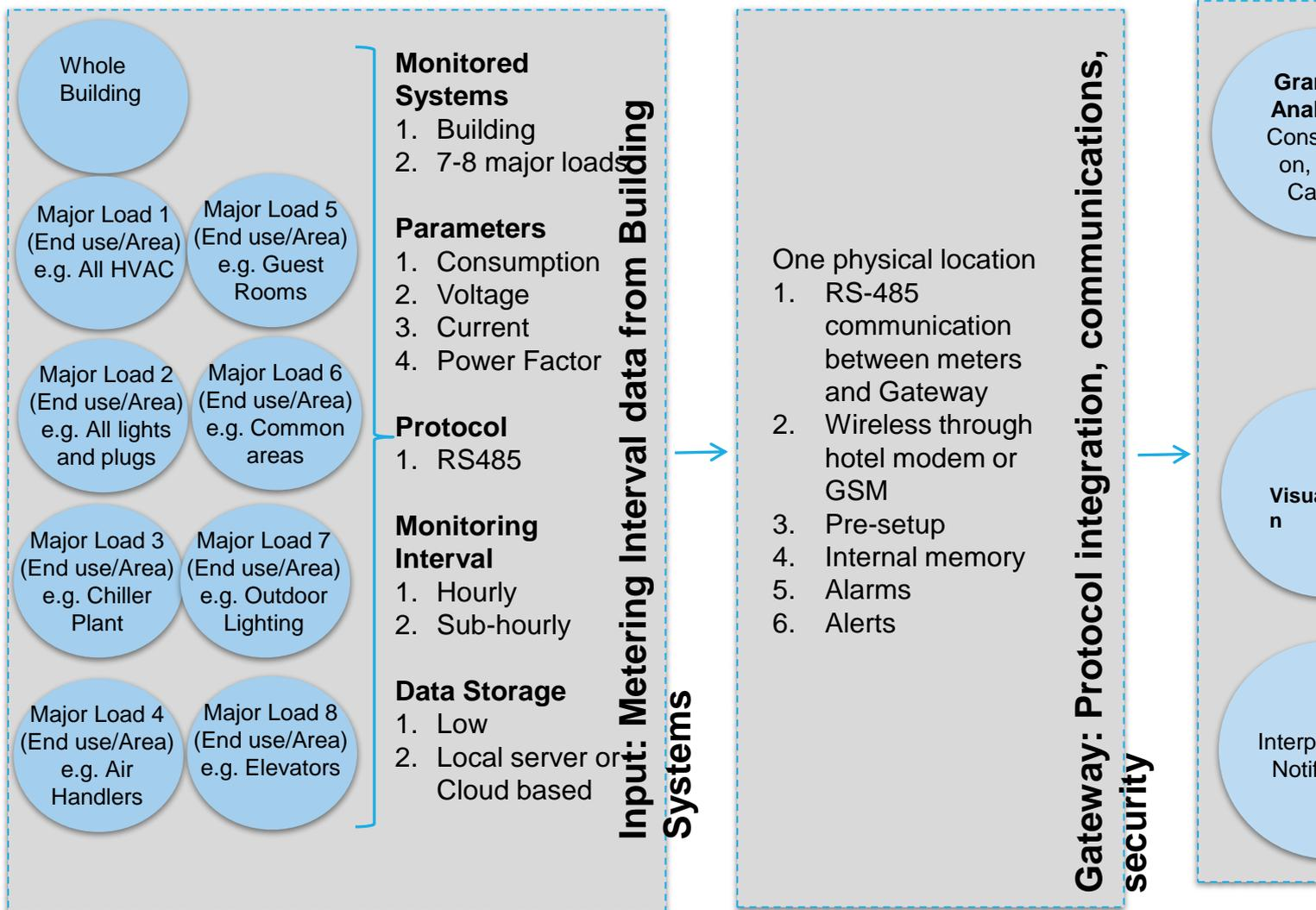
**Figure 1:** Overview of a Hotel EIS Tier 2 Advanced Package. The left column provides the input data from building systems, the middle column provides the gateway integration, communications, security, and the right column provides the visualization and notification.
