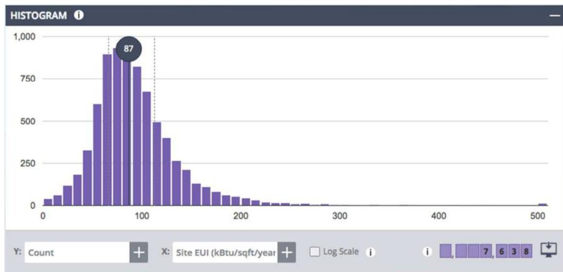
**Figure 3: Screen shot from the Building Performance Database (BPD) for 7,638 U.S. hotels. Median Site EUI is 87 kBtu/sf. 25th, 75th percentiles are 66 and 113 kBtu/sf, respectively. (Source: U.S. DOE, 2016)**
