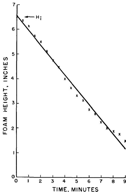
FIG. 2. A foam height-time line showing a typical rate of foam subsidence analysis. The equation from the linear regression analysis is:  $H = 6.55 - 0.596\theta$ . In this case  $R_{t_1}$  is 0.596 in. per minute. Viscosity = 104.5 centipoise. Temperature = 70 F. Run No. FS-9.
