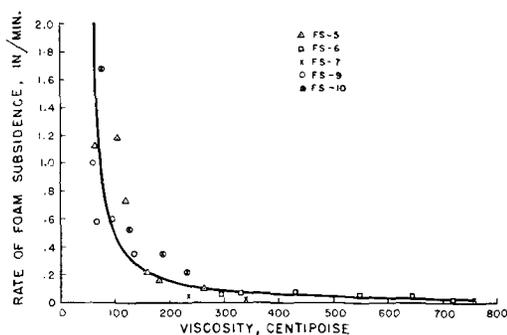
FIG. 4. Rate of foam subsidence as a function of viscosity for whole milk concentrate. The curvilinear regression equation is:
