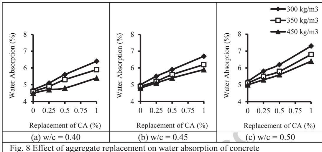
Fig. 8 Effect of aggregate replacement on water absorption of concrete
