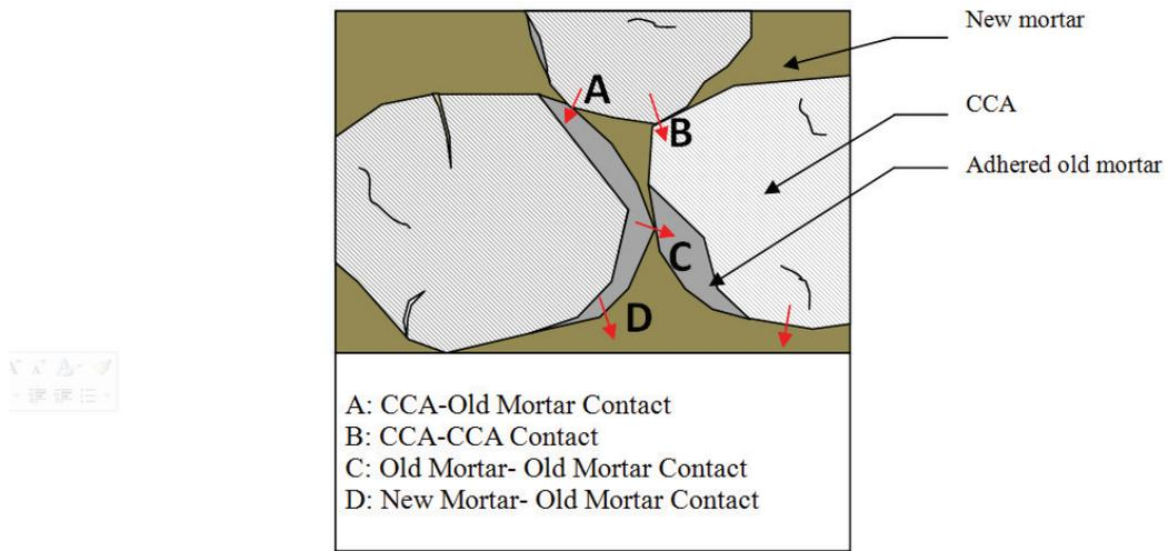
Fig. 4 Load transfer mechanism in CCA concrete
