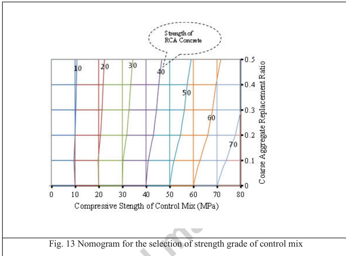
Fig. 13 Nomogram for the selection of strength grade of control mix
