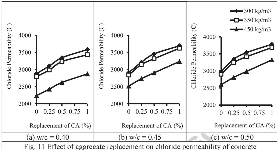
Fig. 11 Effect of aggregate replacement on chloride permeability of concrete
