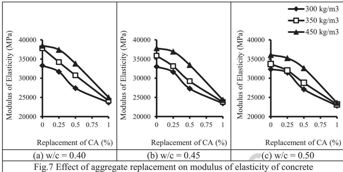
Fig.7 Effect of aggregate replacement on modulus of elasticity of concrete
