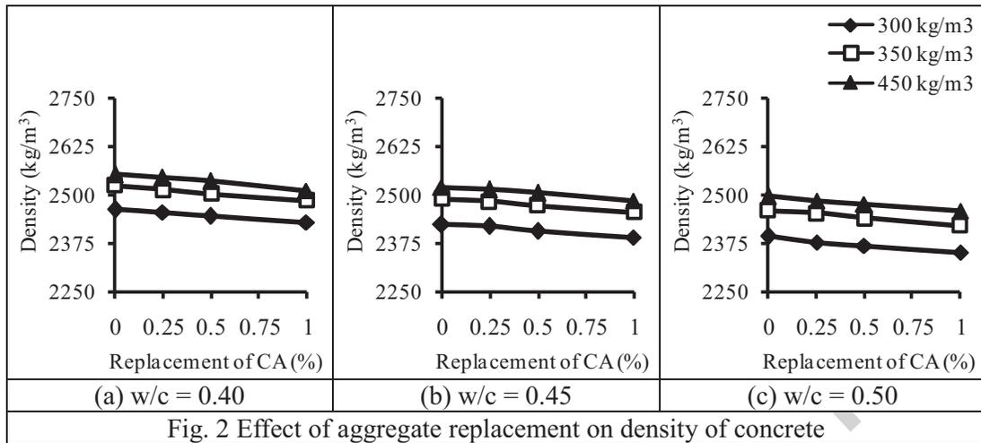
Fig. 2 Effect of aggregate replacement on density of concrete
