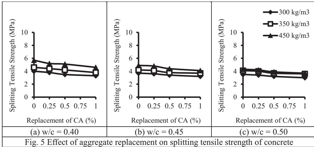
Fig. 5 Effect of aggregate replacement on splitting tensile strength of concrete
