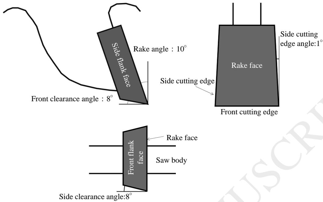
Figure 3 Cutting edge shape
