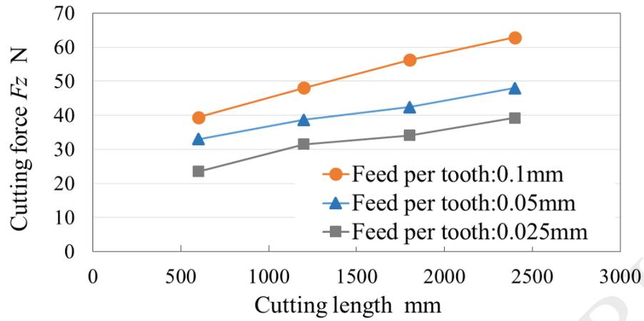
Figure 15 Effect of feed per tooth on cutting force  $F_z$
