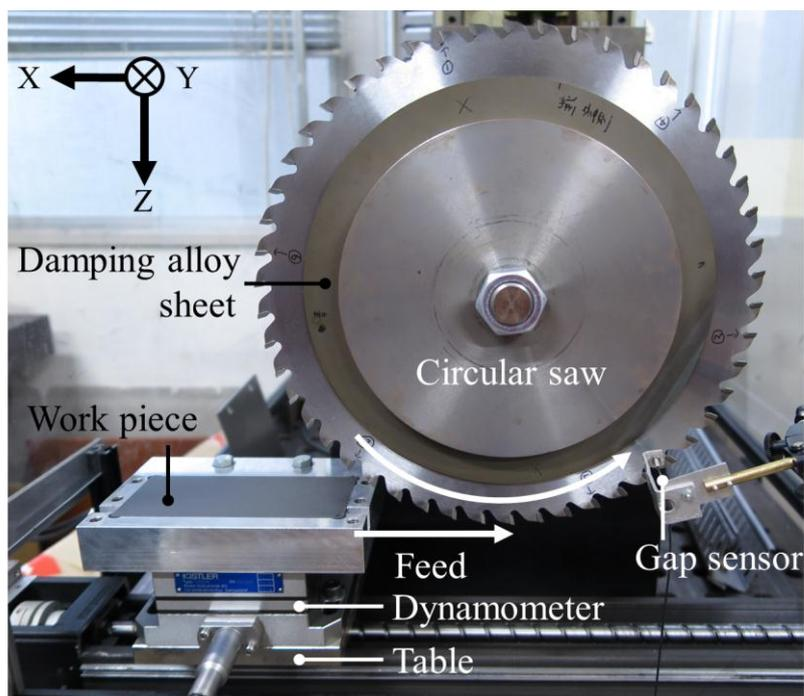
Figure 1 CFRP straight cutting machine using circular saw
