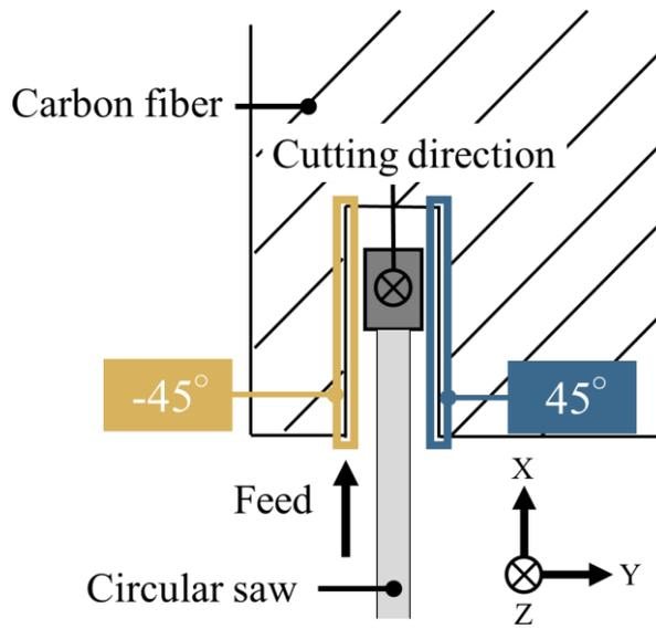
Figure 18 Schematic of circular saw cutting when 45° and -45° carbon fiber is cut
