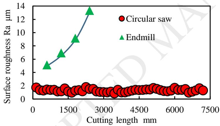
Figure 10 Comparison of surface roughness on circular saw cutting and milling
