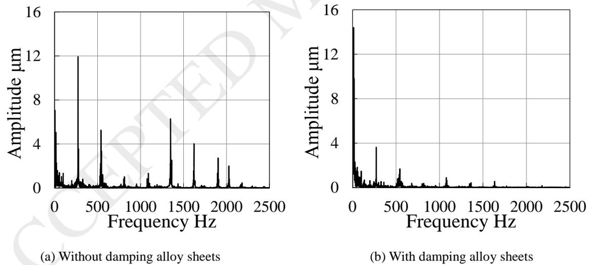
Figure 4 Effect of damping alloy sheet on vibration of circular saw body during cutting
