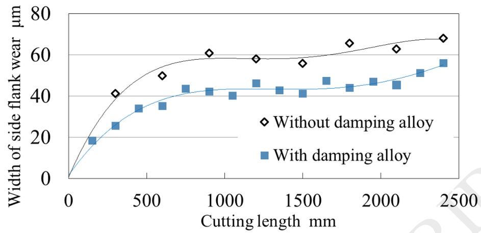
Figure 5 Transition of side flank wear affected by with/without damping alloy
