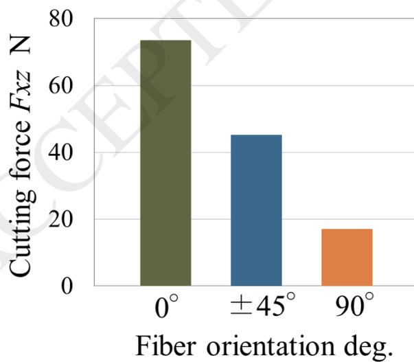
Figure 17 Effect of fiber orientation on cutting force
