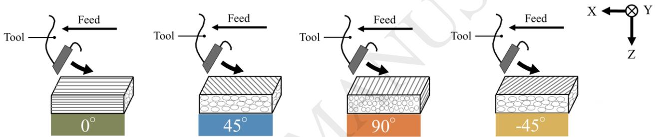
Figure 16 Definition of carbon fiber orientation
