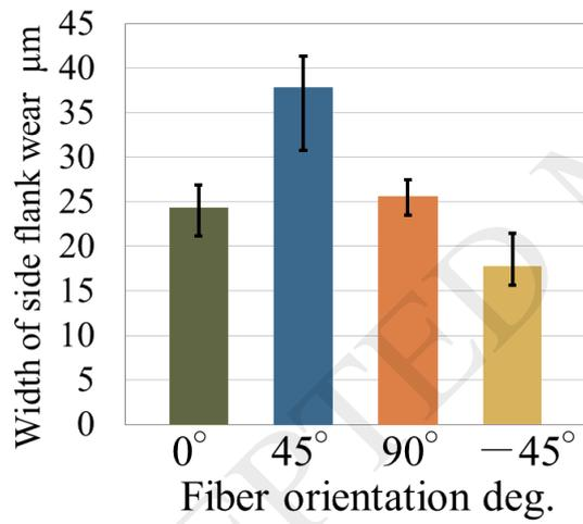
Figure 21 Effect of fiber orientation on side-flank wear
