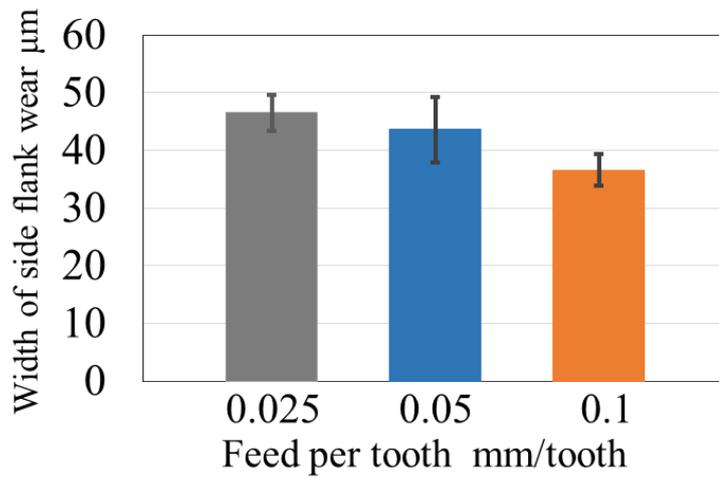
Figure 11 Comparison of average side flank wear affected by feed per tooth
