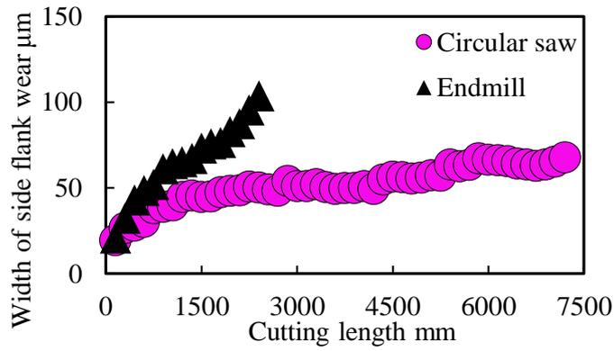
Figure 9 Comparison of flank wear on circular saw cutting and milling
