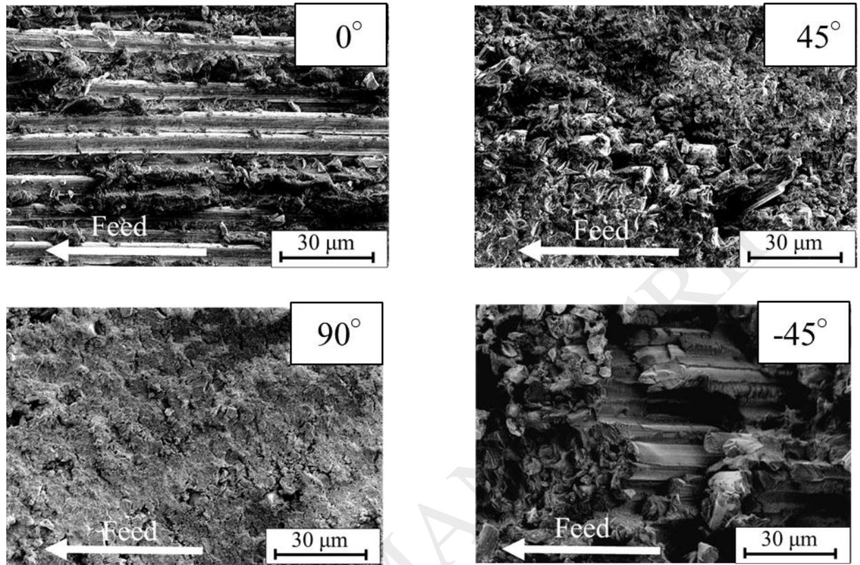
Figure 22 SEM images of machined surface on circular saw cutting
