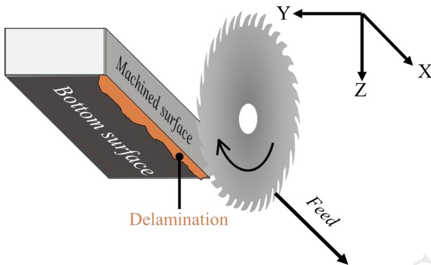
**Figure 13** Delamination area on cutting CFRP by circular saw
