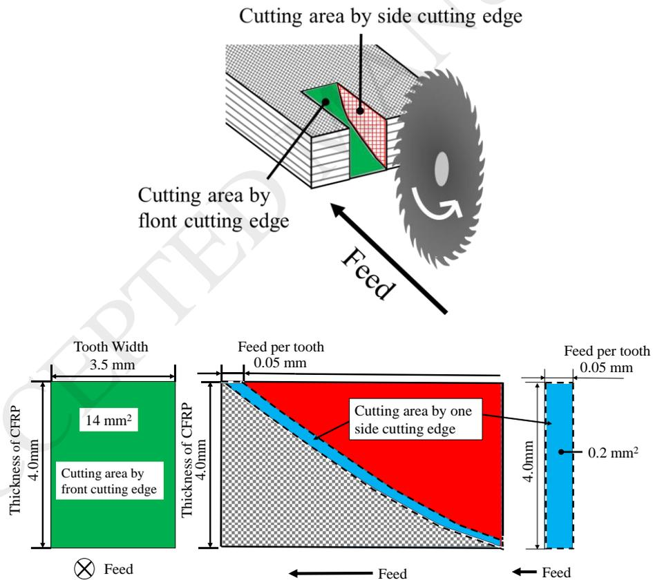
Figure 19 Cutting area by front cutting edge and side cutting edge
