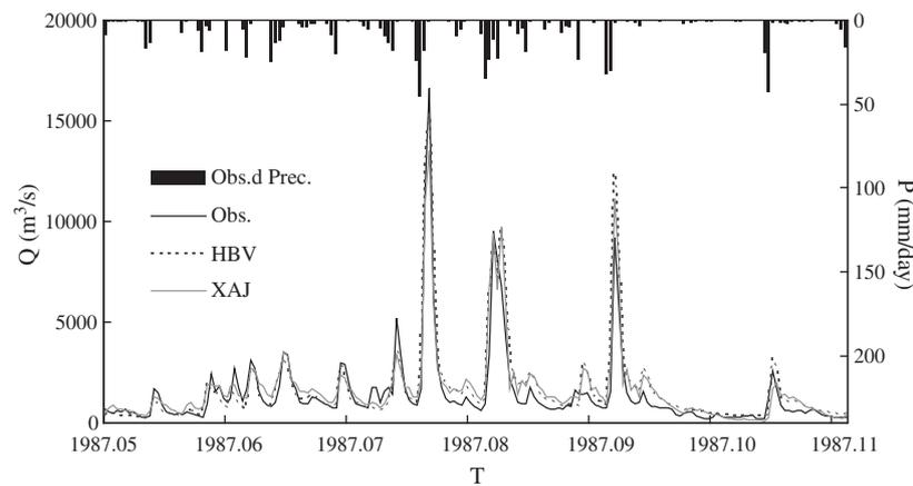
Fig. 4. Observed and simulated discharge hydrograph in the period of May to November in 1987.
