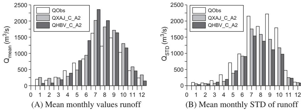
Fig. 6. The comparison of runoff simulation driven by CGCM3 A2 scenario downscaled by SSVM.
