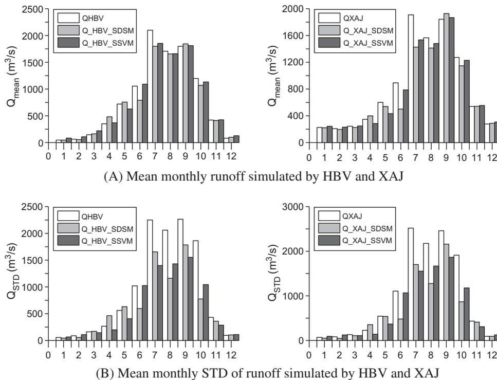
Fig. 5. The comparison of runoff simulation driven by NCEP/NCAR reanalysis data downscaled by SSVM and SDSM.
