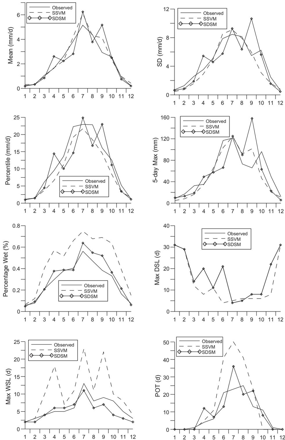
Fig. 3. Comparison of mean monthly rainfall statistics downscaled from NCEP/NCAR reanalysis data using SSVM and SDSM.
