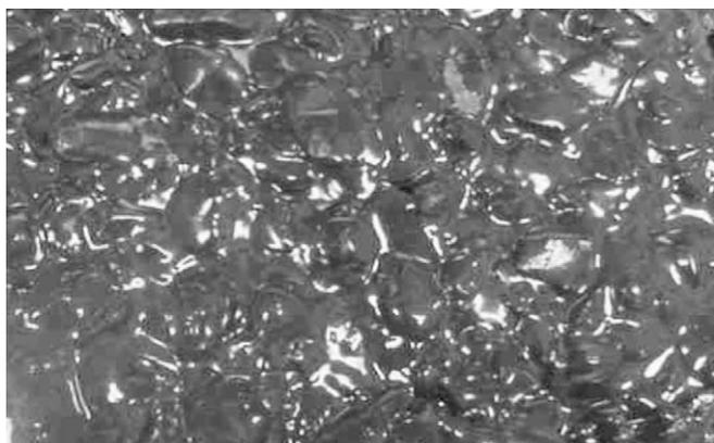
**Fig. 2.** Image of modified gravel covered with molten rubber-modified asphalt; the gravel surface was completely wetted by the asphalt.
