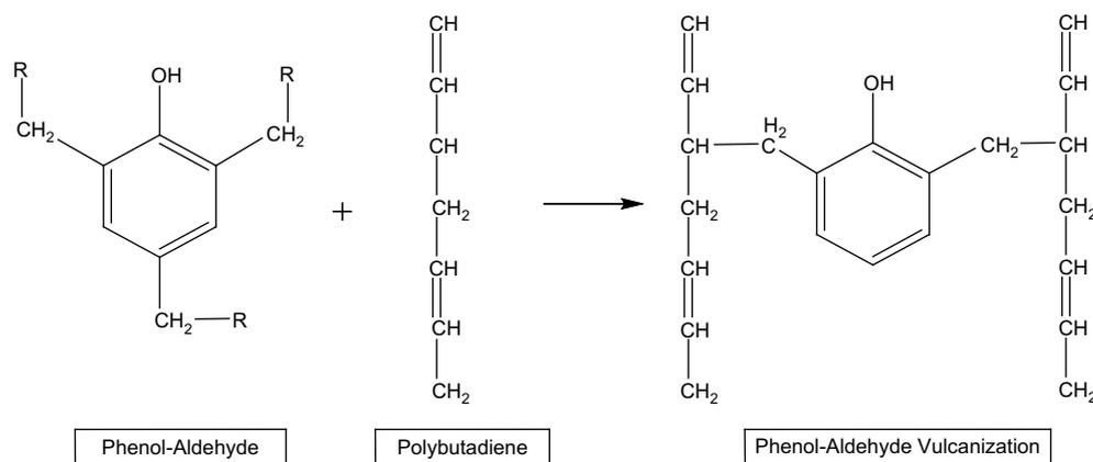
Fig. 1. Chemical reaction between PA resin and polybutadiene.
