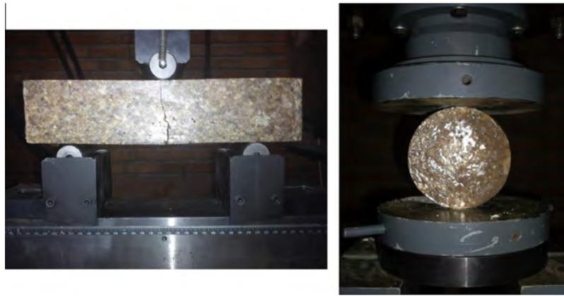
Fig. 3. SENB and BD test setup.
