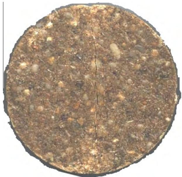
**Fig. 8.** Typical fracture trajectory observed for a BD specimen made of PC material.
