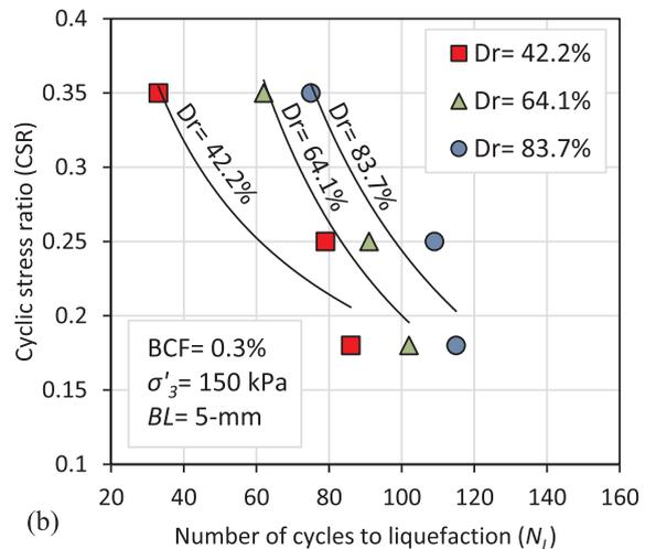
Fig. 8. Effect of relative density on liquefaction resistance of the unreinforced and reinforced specimens at  $\sigma'_3 = 150 \text{ kPa}$  for (a) unreinforced specimen; and (b) reinforced specimens with  $BCF = 0.3\%$ , and  $BL = 5\text{-mm}$ .
