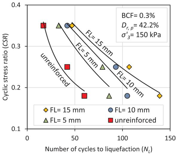
Fig. 7. Effect of BCF length on liquefaction resistance of reference and reinforced specimens for  $BCF = 0.3\%$ ,  $\sigma'_3 = 150 \text{ kPa}$ , and  $D_{r,p} = 42.2\%$ .
