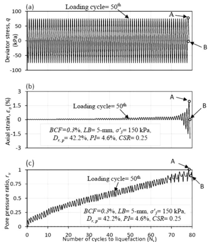
**Fig. 3.** Typical results of the cyclic triaxial test for a reinforced specimen for BCF = 0.3%,  $D_{r,p} = 42.2\%$ , CSR = 0.25, and  $\sigma'_3 = 150$  kPa. (a) Variation of the deviator stress ( $q$ ) with number of cycles to liquefaction ( $N_L$ ); (b) Variation of the axial strain ( $\epsilon_a$ ) with number of cycles to liquefaction ( $N_L$ ); and (c) Variation of the pore pressure ratio ( $r_u$ ) with number of cycles to liquefaction ( $N_L$ ).
