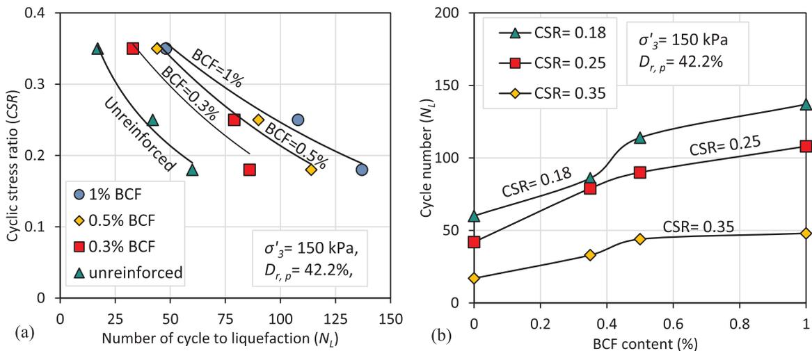
Fig. 6. Effect of BCF contents on liquefaction resistance of reference and reinforced specimens at  $D_{r,p} = 42.2\%$ , and  $\sigma'_3 = 150$  kPa (a) Variations of CSR with  $N_L$ ; (b) Variations of  $N_L$  with BCF contents.
