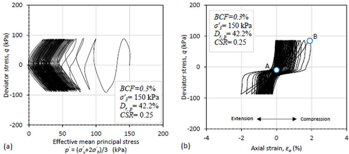
Fig. 5. Typical results of cyclic triaxial test for a reinforced specimen with  $BCF = 0.3\%$ ,  $D_{r,p} = 42.2\%$ ,  $CSR = 0.25$ , and  $\sigma'_3 = 150$  kPa (a) Effective stress path (b) stress-strain relationship (hysteresis loop).
