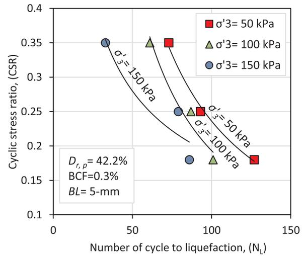
Fig. 9. Effect of effective confining pressure on liquefaction of reinforced specimens when,  $BCF = 0.3\%$ ,  $BL = 5\text{-mm}$ , and  $D_{r,p} = 42.2\%$ .
