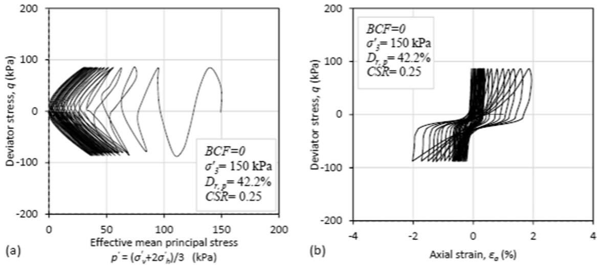
Fig. 4. Typical results of cyclic triaxial test for an unreinforced specimen with  $D_{r,p} = 42.2\%$ ,  $CSR = 0.25$ , and  $\sigma'_3 = 150$  kPa (a) Effective stress path; (b) stress-strain relationship (hysteresis loop).
