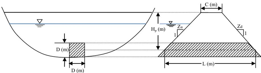
**Fig. 3** Schematic of piping hole (State of Colorado Department of Natural Resources Division of Water Resources 2010)
