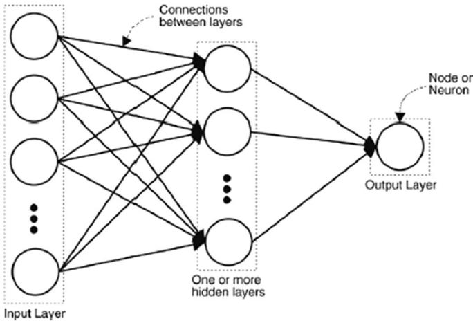
**Fig. 13** Artificial neural network architecture (Gibbs et al. 2006)
