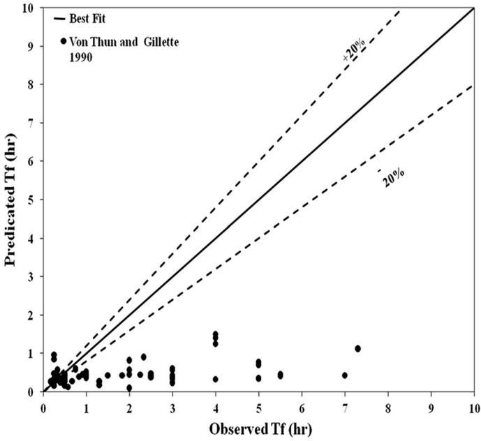
Fig. 9 Performance of Eq. (8) for dam failure time estimation
