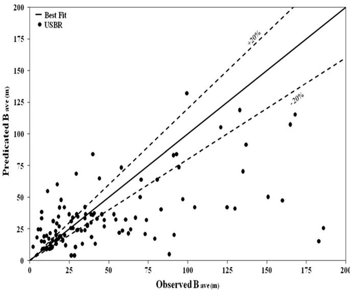
**Fig. 4** Performance of Eq. (3) for dam breach width estimation
