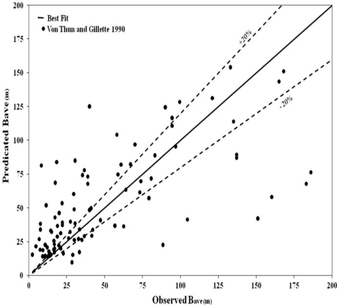
**Fig. 5** Performance of Eq. (4) for dam breach width estimation
