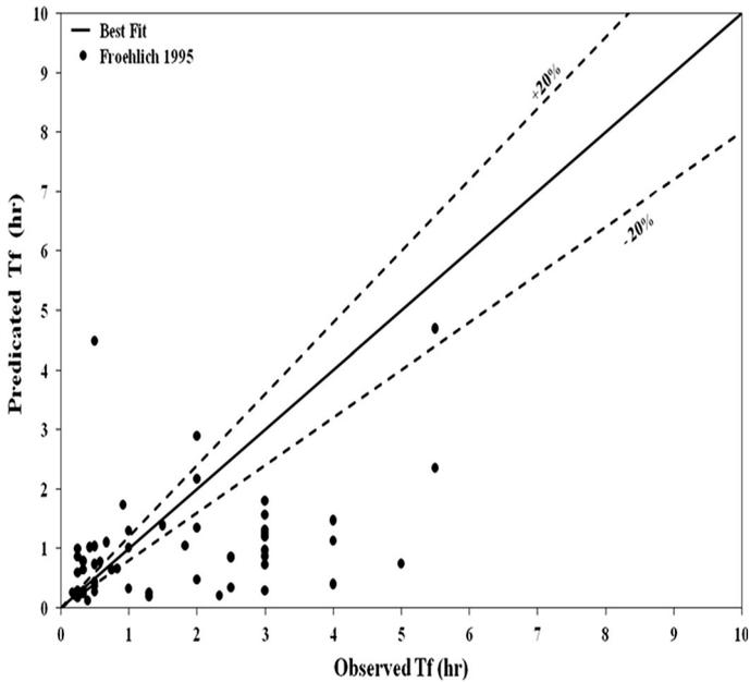
Fig. 10 Performance of Eq. (9) for dam failure time estimation
