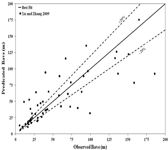
Fig. 8 Performance of Eq. (7) for dam breach width estimation
