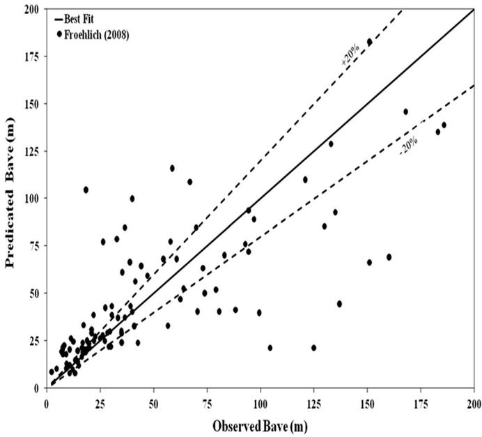
Fig. 7 Performance of Eq. (6) for dam breach width estimation
