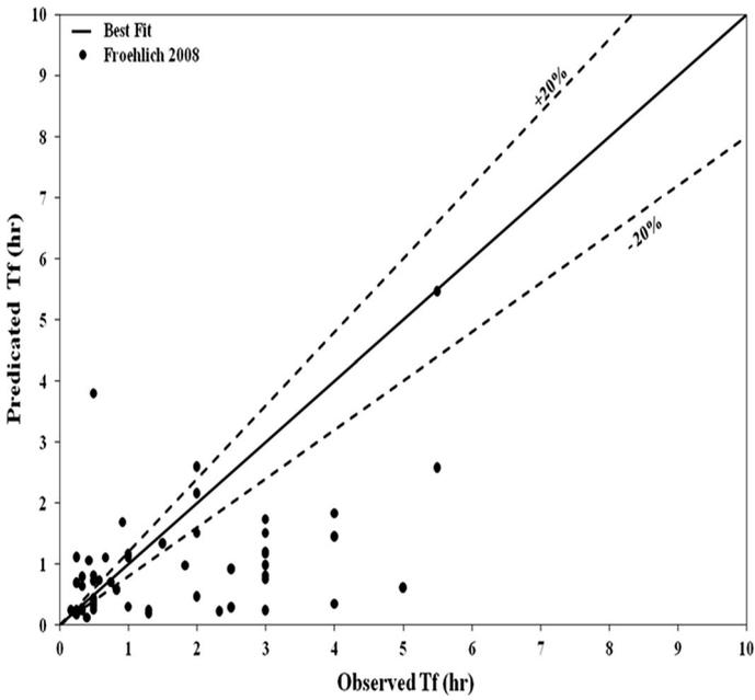
**Fig. 11** Performance of Eq. (10) for dam failure time estimation
