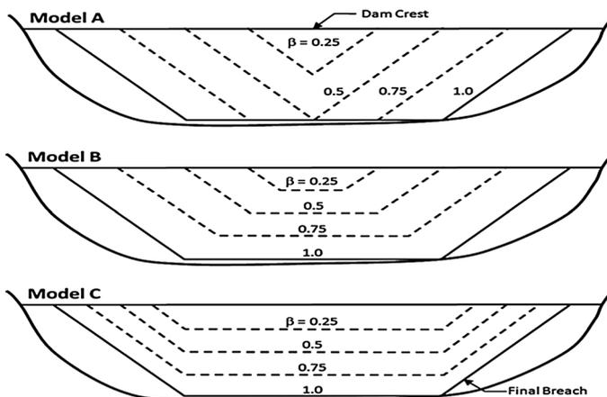
**Fig. 2** Models of breach development (Froehlich 2008)
