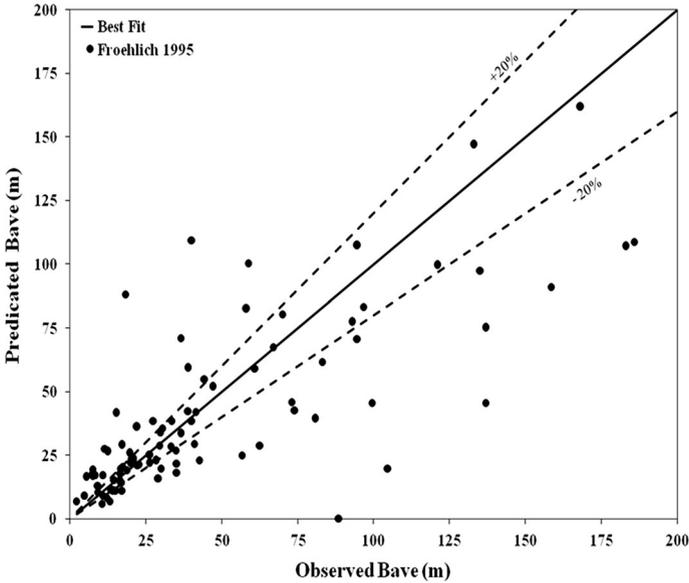
**Fig. 6** Performance of Eq. (5) for dam breach width estimation
