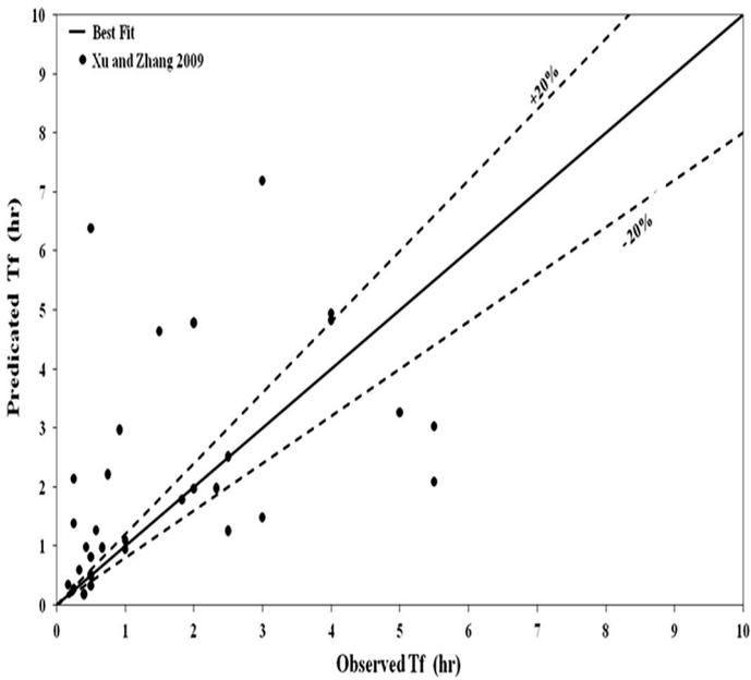
**Fig. 12** Performance of Eq. (11) for dam failure time estimation
