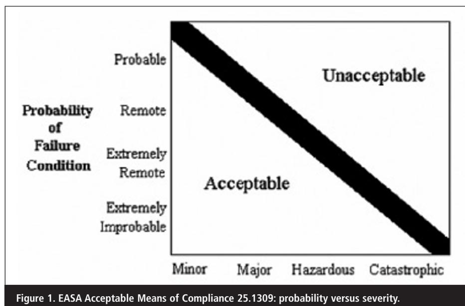
Figure 1. EASA Acceptable Means of Compliance 25.1309: probability versus severity.
