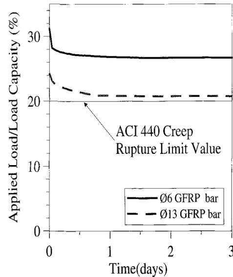
Fig. 7—Load relaxation of GFRP bars
