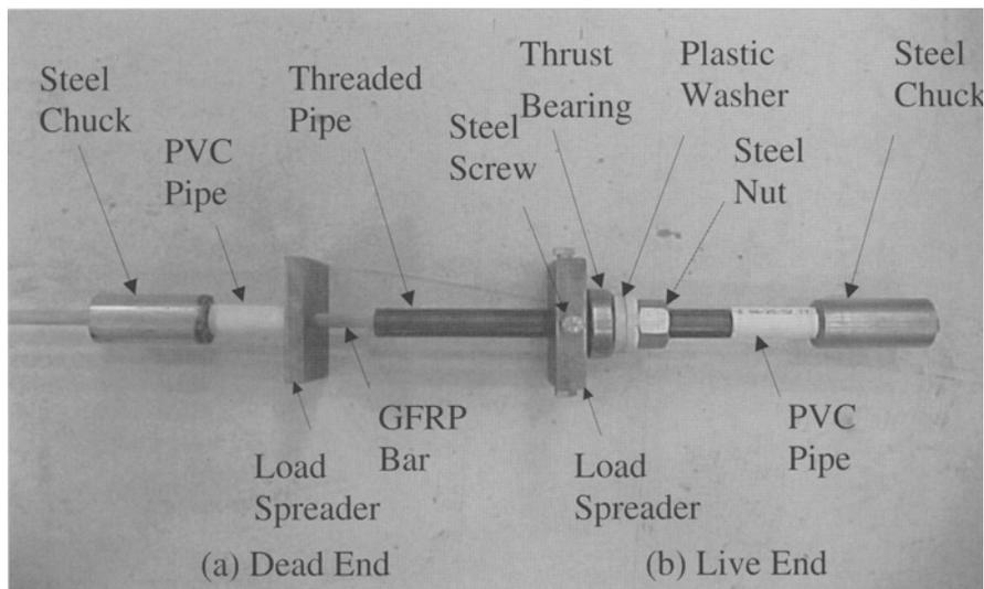
Fig. 1—Hand-held device components
