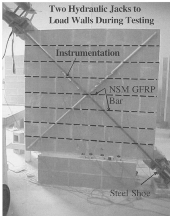
Fig. 8—Testing of retrofitted masonry walls with prestressed NSM GFRP bars
