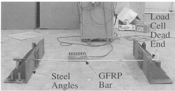
Fig. 6—Test setup for component evaluation
