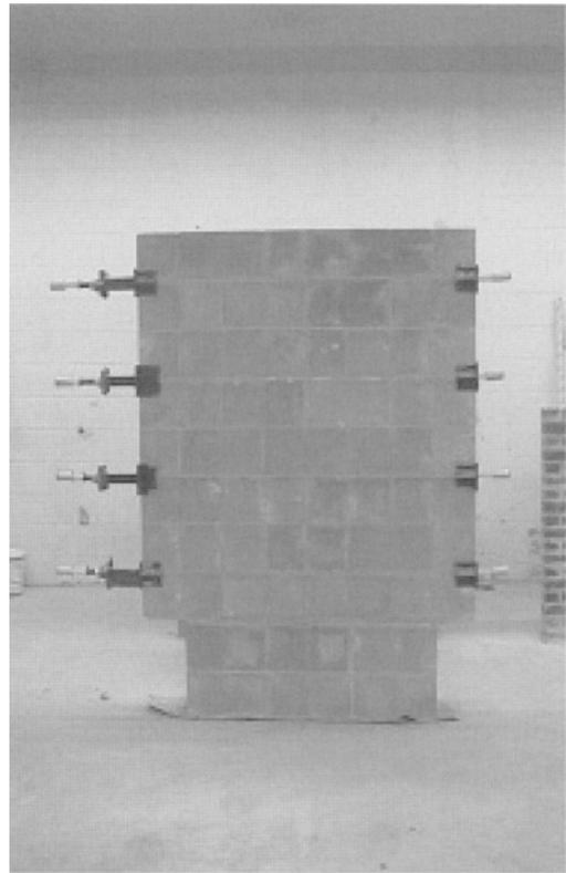
Fig. 5—Assembled system in a masonry wall
