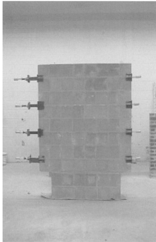
Fig. 5—Assembled system in a masonry wall
