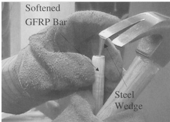
Fig. 3—Inserting steel wedge in a GFRP bar
