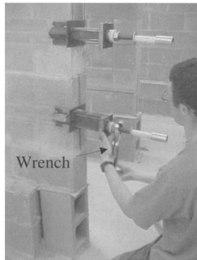
Fig. 4—Manually stressing a GFRP bar with a wrench
