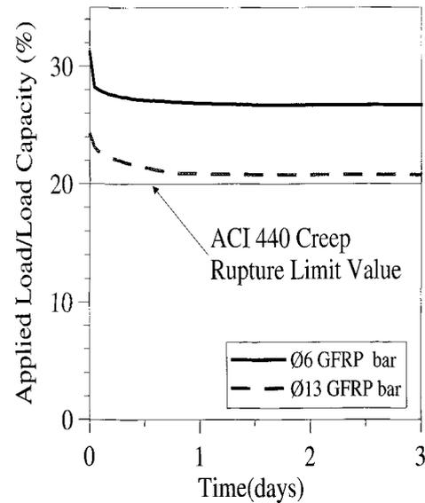
Fig. 7—Load relaxation of GFRP bars
