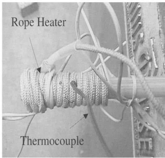
Fig. 2—Heating of a GFRP bar
