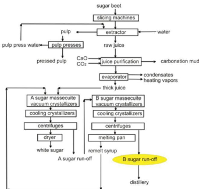
Fig. 1. Simplified scheme of the sugar technology completed with fermentation
