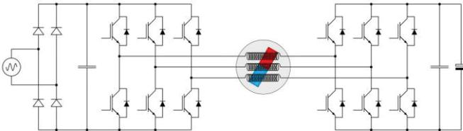
Figure 3: AC dual-inverter topology with isolated DC links
