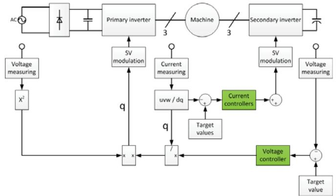
Figure 4: Dual-inverter control scheme
