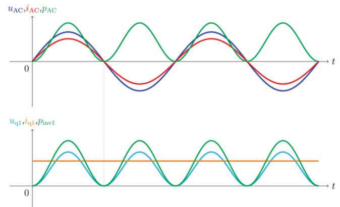
Figure 5: Exemplary progressions of voltage, current and power at AC input and primary inverter output
