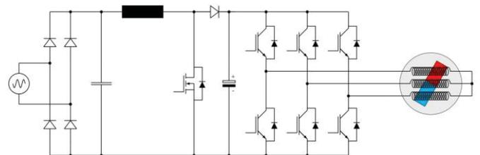
Figure 1: Example for AC inverter with active PFC stage
