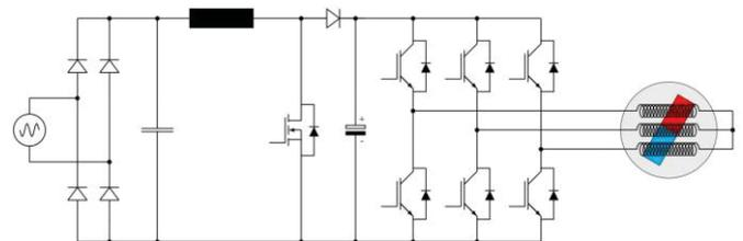
Figure 1: Example for AC inverter with active PFC stage
