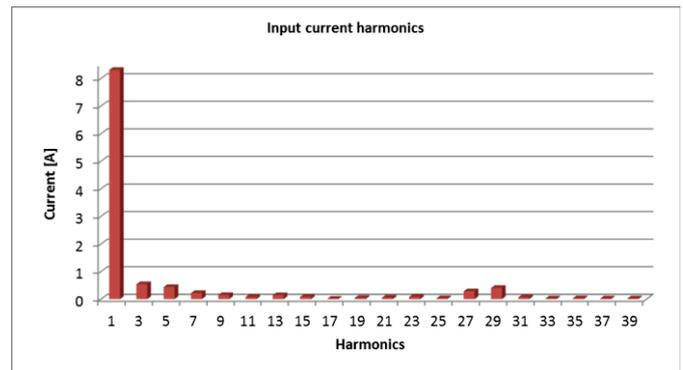
Figure 8: Harmonics of input current at operating point
