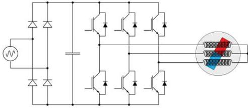
Figure 2: AC inverter with small film capacitor
