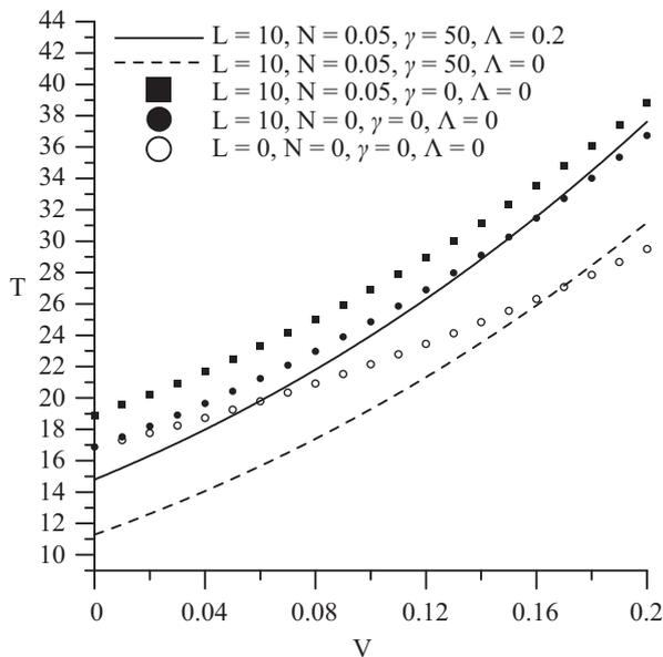
Fig. 3 Mean squeeze film time  $T$  versus concentration parameter  $V$  for different  $L$ ,  $N$ ,  $\gamma$  and  $\Lambda$ .
