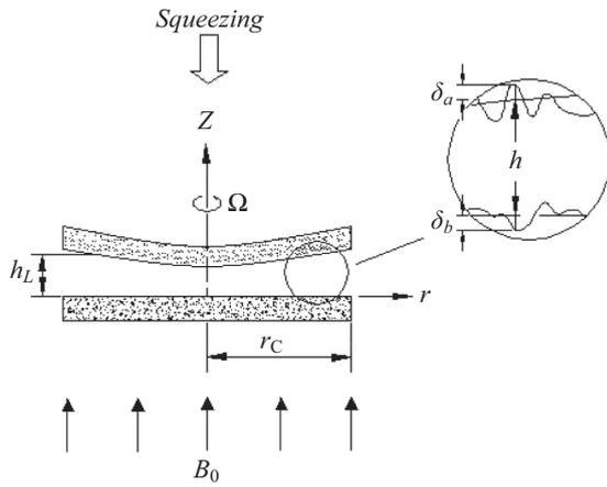
Fig. 1 Squeeze film geometry of rotational rough curved circular disks lubricated with a non-Newtonian ferrofluid.
