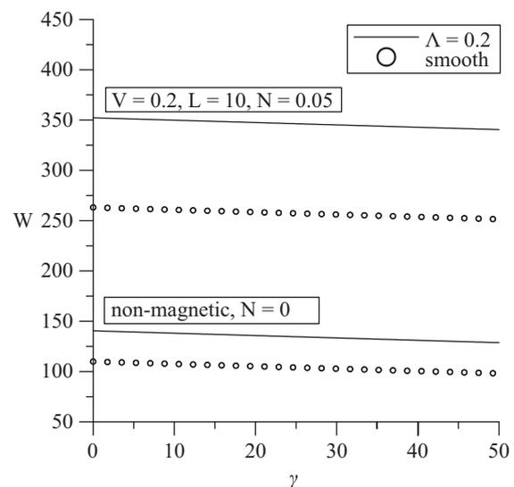
Fig. 2 Mean load capacity  $W$  versus rotational parameter  $\gamma$  for different  $V$ ,  $L$ ,  $N$  and  $\Lambda$ .
