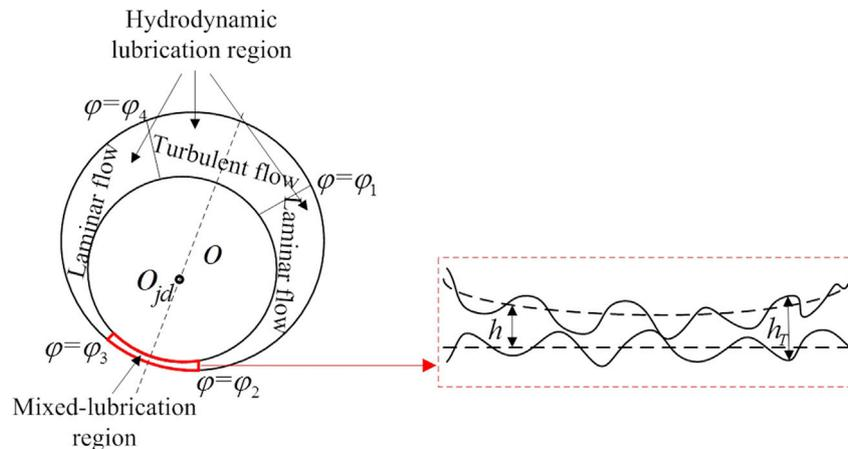
Fig. 2. Geometry model of bearing including asperity contact and turbulence.
