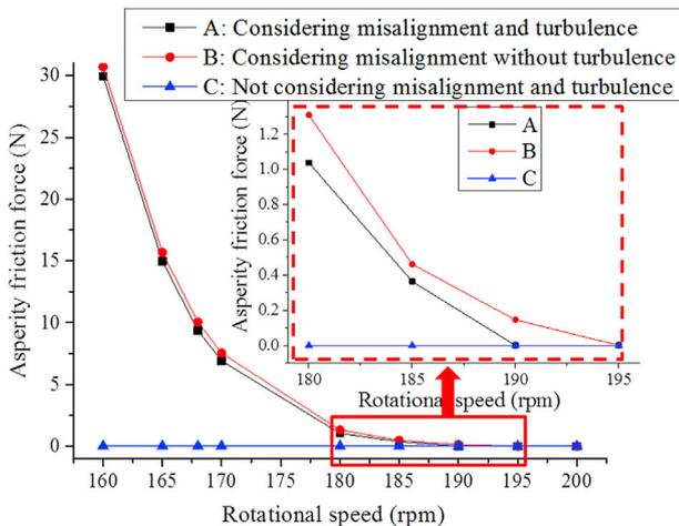
Fig. 9. Asperity friction force versus speed for the different models.
