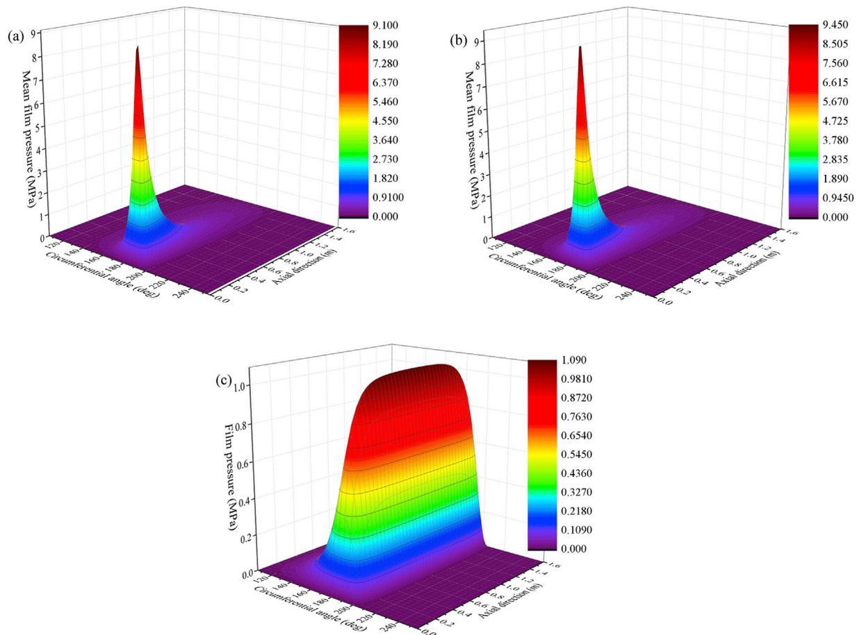
Fig. 5. Mean hydrodynamic pressure distribution at rotational speed of 190 r/min: (a) Considering turbulence and journal misalignment; (b) Considering journal misalignment without turbulence; (c) Not considering journal misalignment and turbulence.
