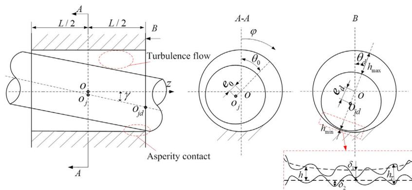
Fig. 1. Geometry model of the misaligned journal bearing.
