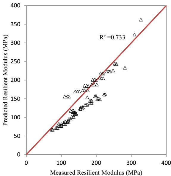
Fig. 5. Measured resilient modulus from tests versus predicted resilient modulus from Eq. (9).
