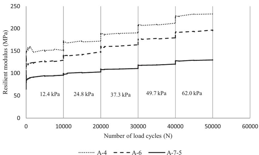
Fig. 3. Resilient modulus values vs. number of load repetitions for different deviatoric stress levels for stabilised soils.
