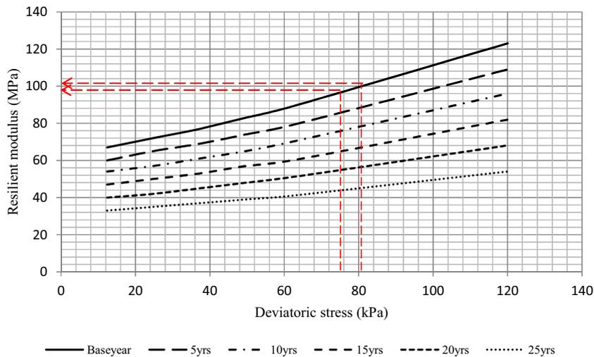
**Fig. 7.** Iteration analysis of resilient modulus and deviatoric stress convergence for soil A-7-5 stabilised with 2%CC and for five stages of 5 years each.
