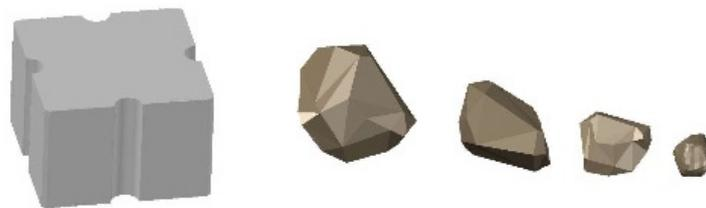
Fig. 1 Virtual 3D models of stones and antifer.
