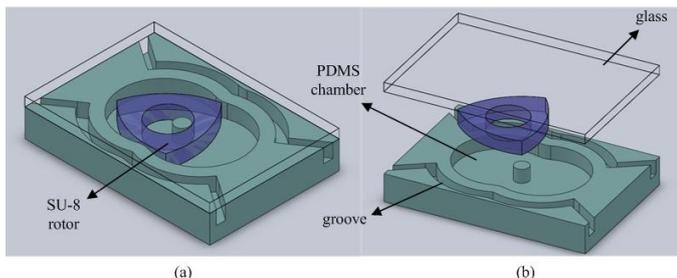
Fig. 4. Three dimensional diagram of the small Wankel engine.
