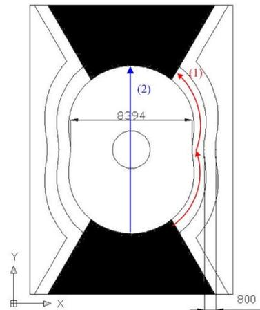
Fig. 3. Schematic diagrams of the small Wankel engine (unit:  $\mu\text{m}$ ).
