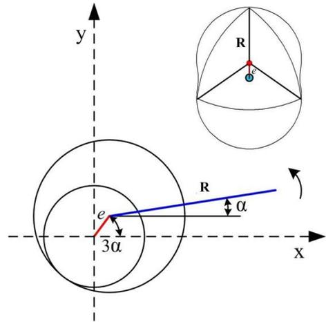
Fig. 1. The epitrochoid contour of Wankel engine.
