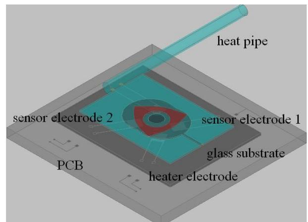
Fig. 8. The modified package of the small Wankel engine.
