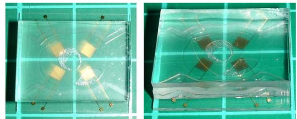
Fig. 7. A fabricated small Wankel engine ( $R=4990\mu\text{m}$ ).
