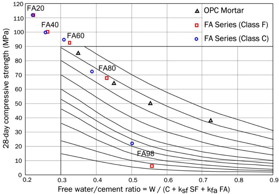
Fig. 8. Compressive strength vs free water/cement ratio of concrete.
