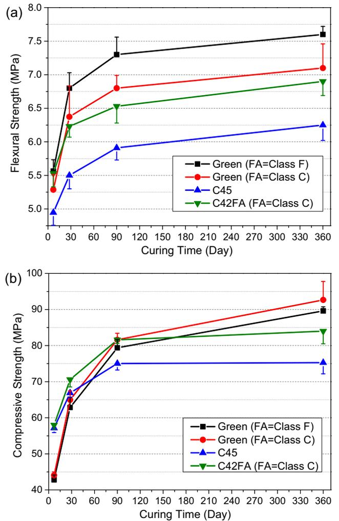
Fig. 10. Mechanical properties of Concrete series.
