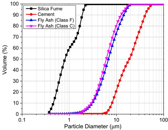
Fig. 3. Particle size distribution of cement, fly ash and silica fume.
