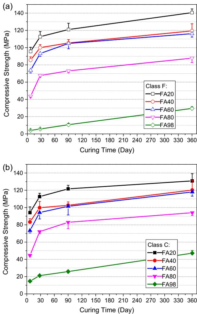
Fig. 7. Compressive strength development of Mortar-FA series.
