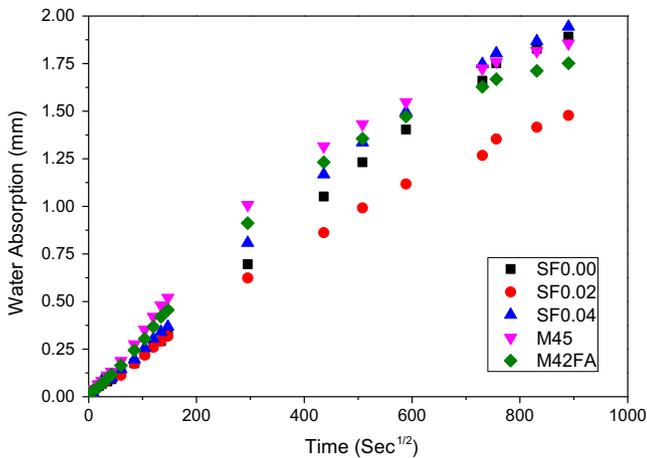
Fig. 5. Water absorption of Mortar-SF series.
