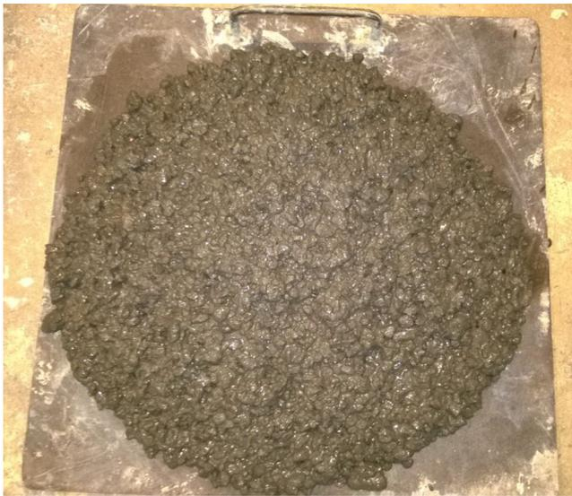
Fig. 9. Slump test of fresh green concrete.
