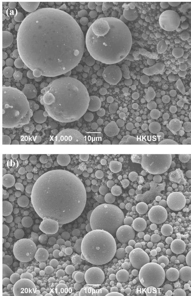
Fig. 2. SEM images of fly ash.
