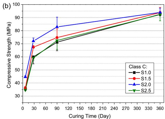
Fig. 6. Compressive strength development of Mortar-S series.
