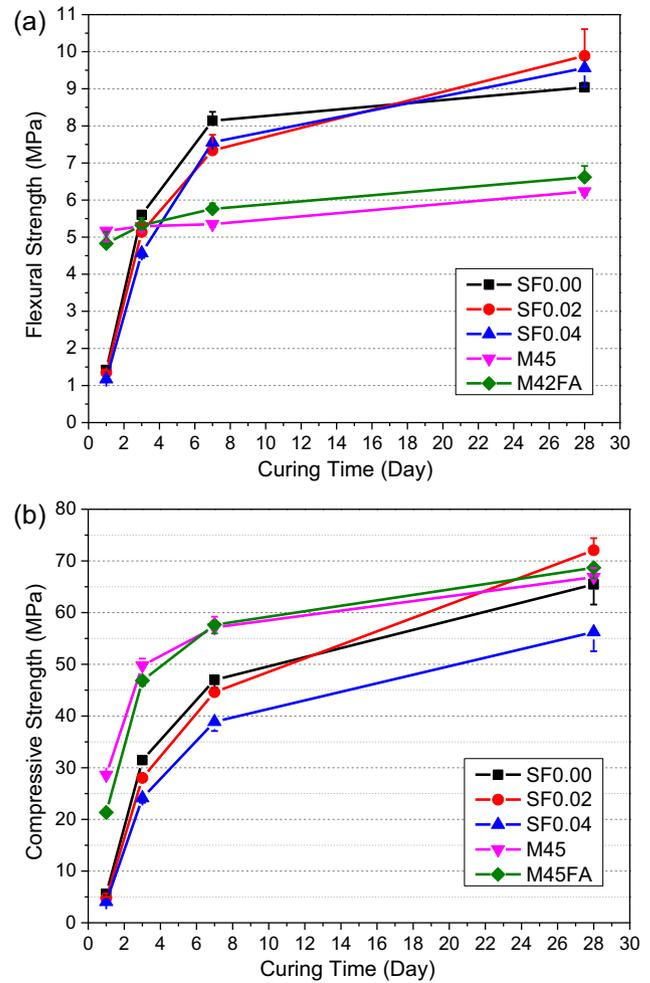
Fig. 4. Mechanical properties of Mortar-SF series.
