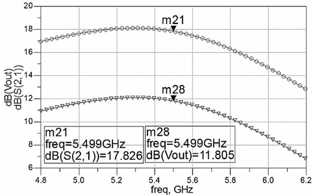
Fig.11: Voltage and power gain of LNA
