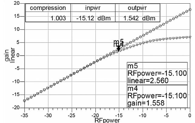
Fig.8: 1dB-compression point of the LNA.
