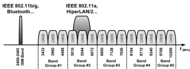
Fig.1: Frequency allocation of MB-OFDM UWB channels [4].
