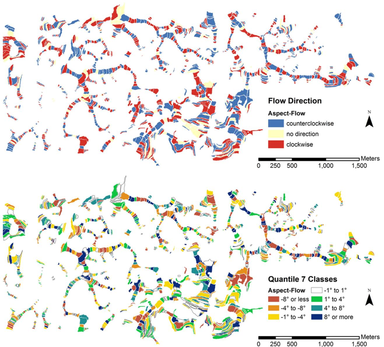
**FIGURE 7.** This figure shows the valley terrace orientations according to the terrace flow analysis outlined in this paper. The terraces have been classified into clockwise and counterclockwise flow (top) and 7 classes (bottom) to indicate the degree of difference in flow direction.
