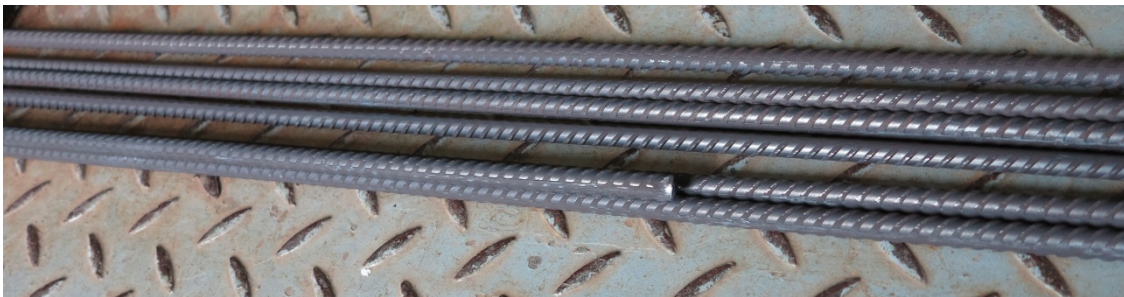
Figure 19: Ribbed Fe-SMA bars with a diameter of 8 mm that can be utilized for concrete reinforcement.
