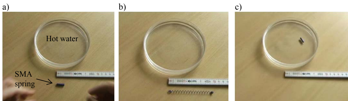
Figure 1: a) SMA spring and a dish of warm water, b) the spring strongly deformed, c) the spring ‘remembering’ its former shape when exposed to elevated temperature.
