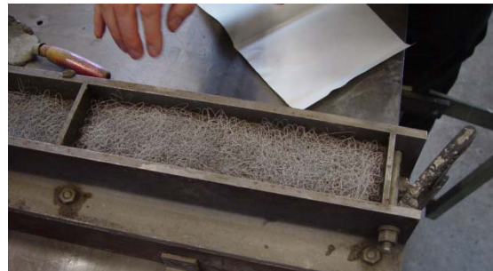
Figure 10: Mixing of the short NiTi fibers with mortar in a prism formwork.
