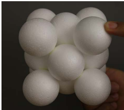
Figure 3: Crystal lattice face-centered-cubic (fcc) model of the austenite \gamma -phase.
