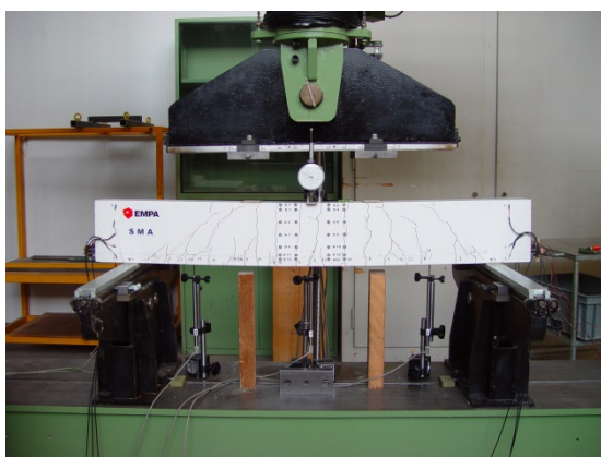
Figure 5: Concrete beam reinforced with NiTi wires and testing set-up for loading.
