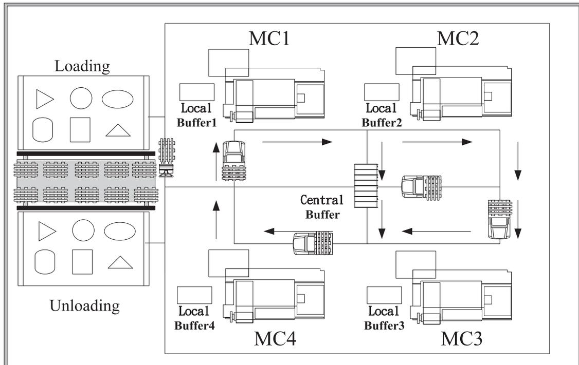
Fig. 1. Layout of the FMS in this study.
