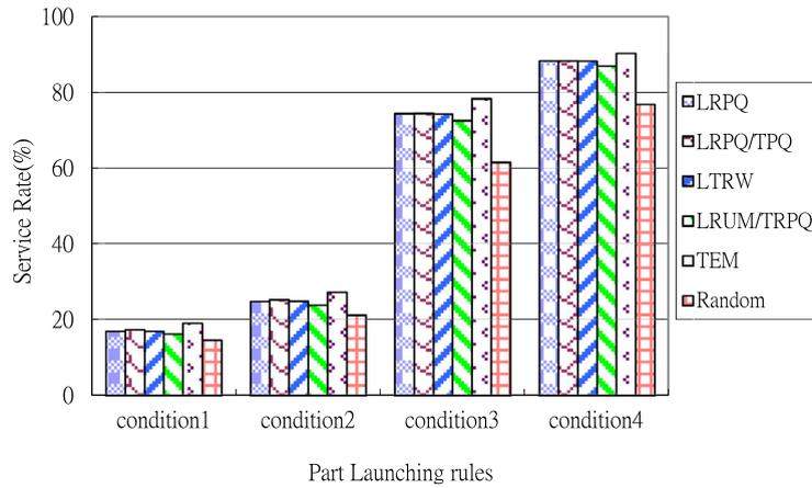
Fig. 4. Service rate measure for part launching rules.
