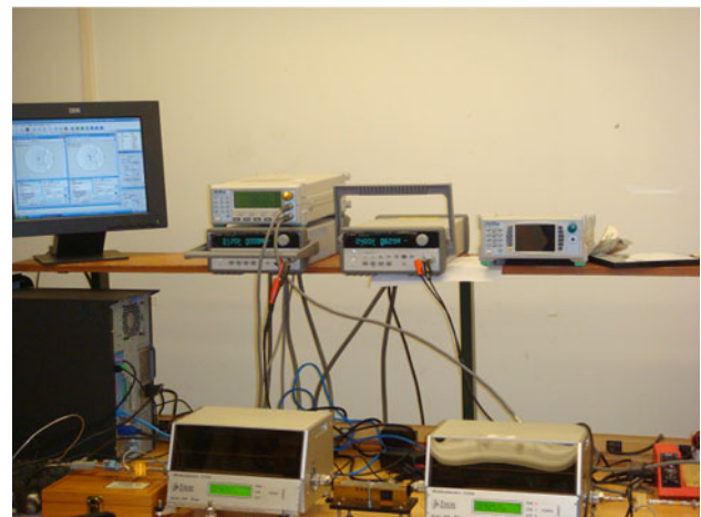
Fig. 7 Load-pull bench used to characterize the device
