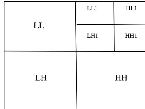
**Fig 1: Two level DWT decomposition**
