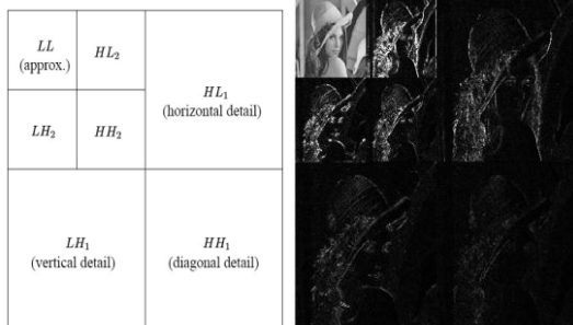
2.(a): Decomposition Structure (b) Decomposed Image
