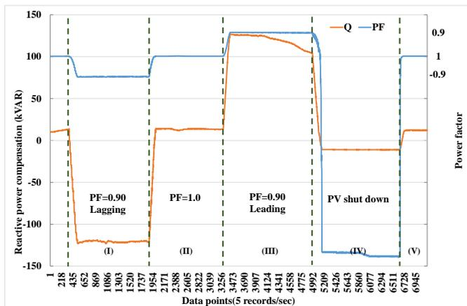
Fig. 8. Profiles of reactive power compensation and power factor (2015/06/25-10 : 30AM).
