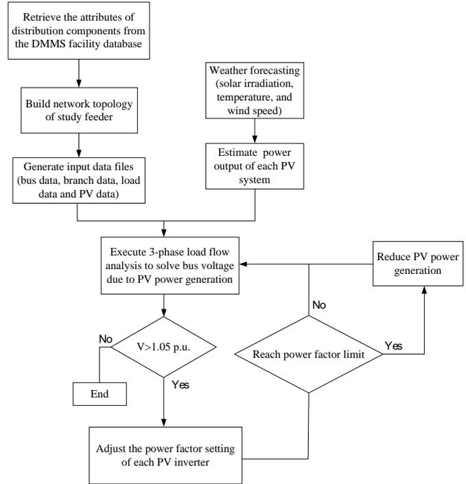
Fig. 5. Decision making process of power factor setting and real power curtailment for control of PV smart inverters.
