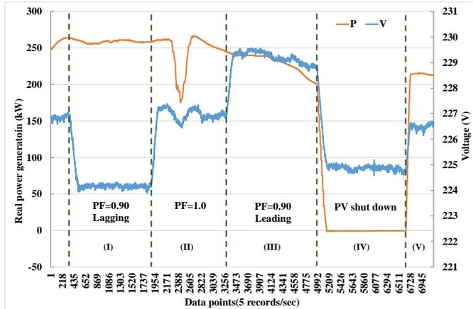
Fig. 7. Profiles of real power generation of PV system and PCC voltage after control of smart inverter (2015/06/25-10 : 30AM).
