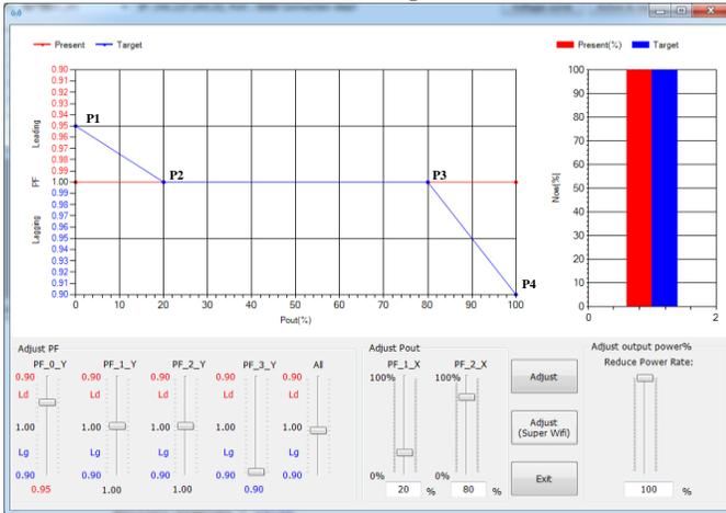
Fig. 4. Array setting of Watt-Power factor for control of a smart inverter.
