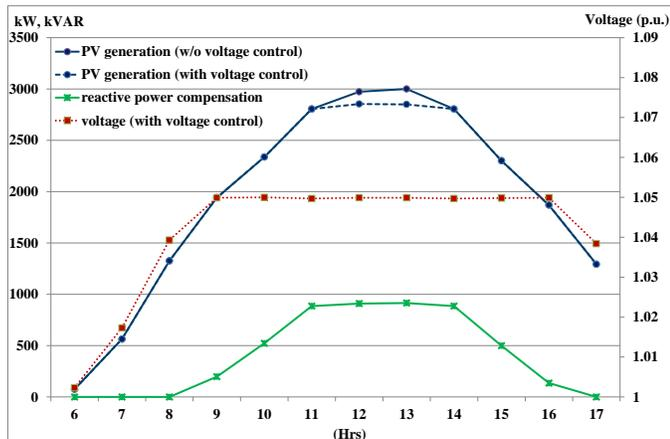
Fig. 11. Profiles of real power generation, reactive power compensation and bus voltage of test PV farm (using smart inverter).
