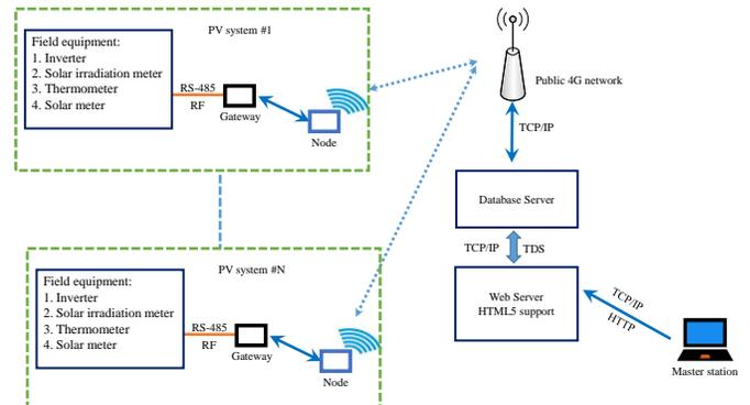
Fig. 3. Communication topology of REMS.
