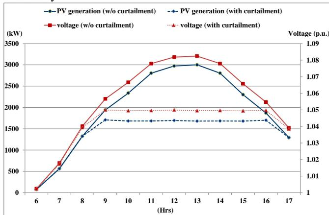
Fig. 10. Profiles of real power generation and bus voltage of test PV farm (using real power curtailment).
