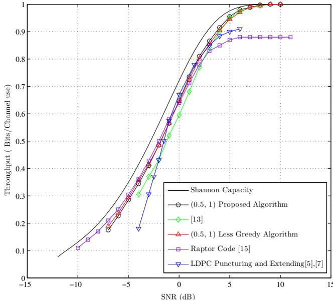
Fig. 5. Throughput comparison of the proposed IR-HARQ scheme with other alternatives.
