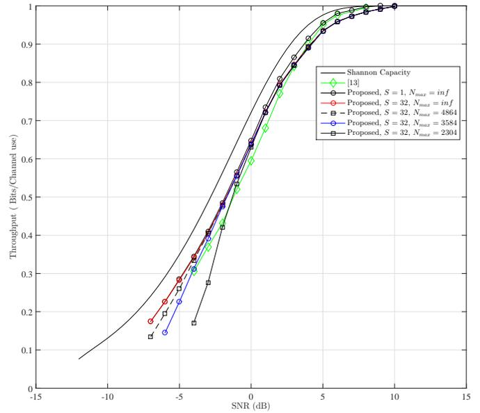
Fig. 6. Throughput of the proposed system for different number of decodings with a cluster size of  $S = 32$ .
