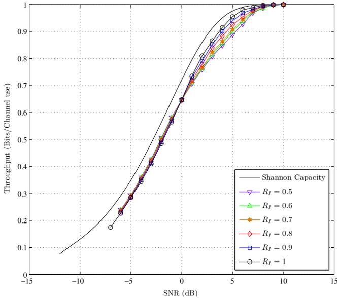
Fig. 4. Throughput of the proposed IR-HARQ scheme with the proposed puncturing and extending algorithm with different  $R_I$ 's, with  $R_M = 0.5$ .
