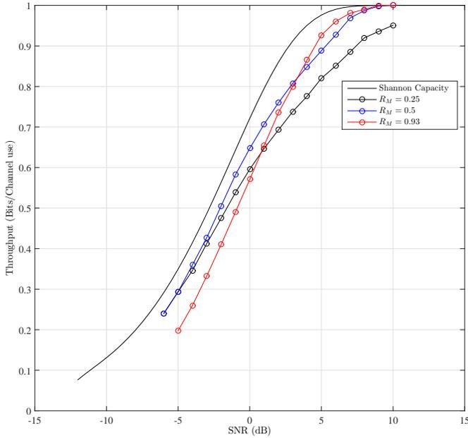
Fig. 3. Throughput of the proposed IR-HARQ scheme with the proposed puncturing algorithm for different  $R_M$ , all with  $R_I = R_M$ .
