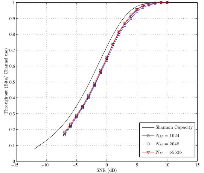
Fig. 7. Throughput of the proposed IR-HARQ scheme for different lengths of the mother polar code, with  $R_M = 0.5$  and  $R_I = 1$ .
