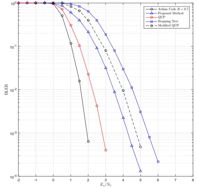
Fig. 2. The BLERs of punctured polar codes with different puncturing algorithms.
