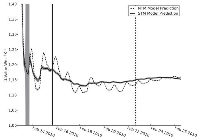
**Fig. 2.** The evolution of estimated U-values as a function of the amount of data used for the NTM model (dashed line) and the STM model (solid line). The magnitude of the statistical error is also shown as a shaded band around each line. This error reduces to very small values after a very short period of time. The vertical lines indicate the first time that the previous 24 h of U-values are within  $\pm 1\%$  of the present U-value: 10 days for the NTM model and 3 days for the STM model.
