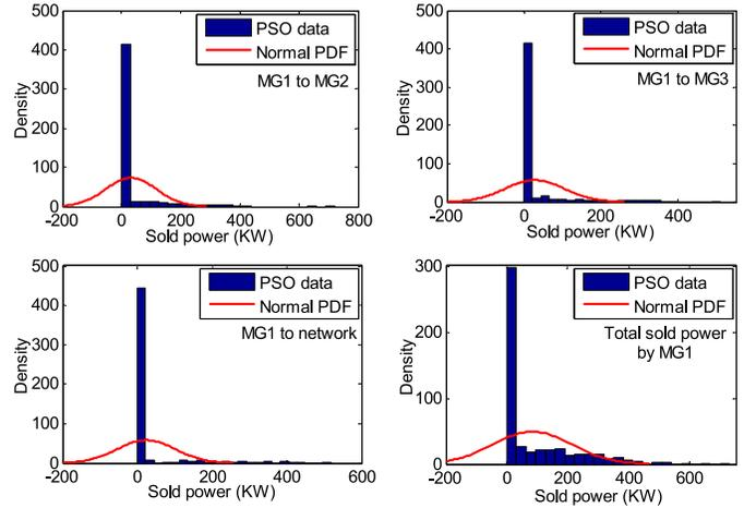
Fig. 10. PDF of sold power in different states of MG1 in interconnected MMG mode.
