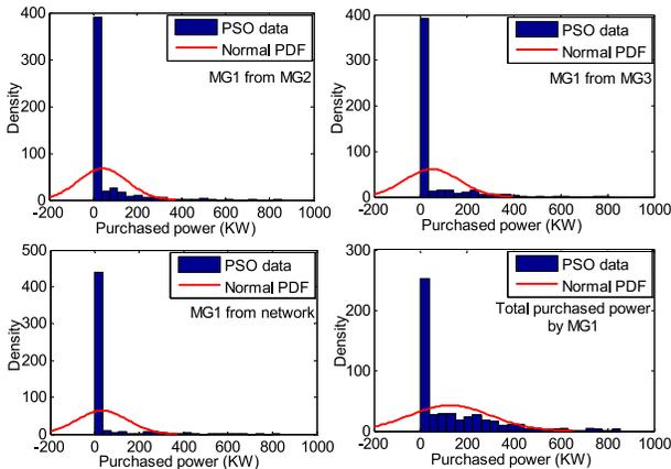
Fig. 9. PDF of purchased power in different states of MG1 in interconnected MMG mode.
