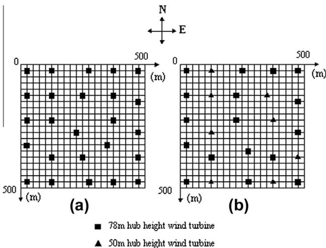
Fig. 9. Optimal layouts generated by GA in third case study: (a) using 78 m hub height wind turbines, (b) using 78 m and 50 m hub heights wind turbines.
