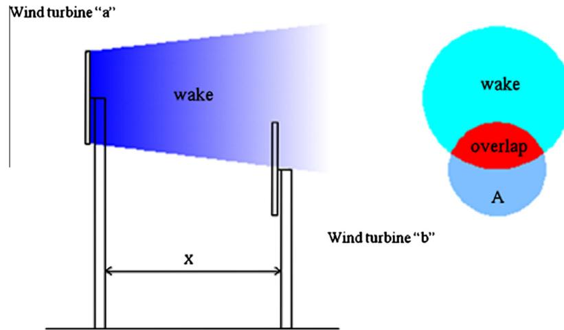
Fig. 1. Schematic of a wake model involving wind turbines with different hub heights.
