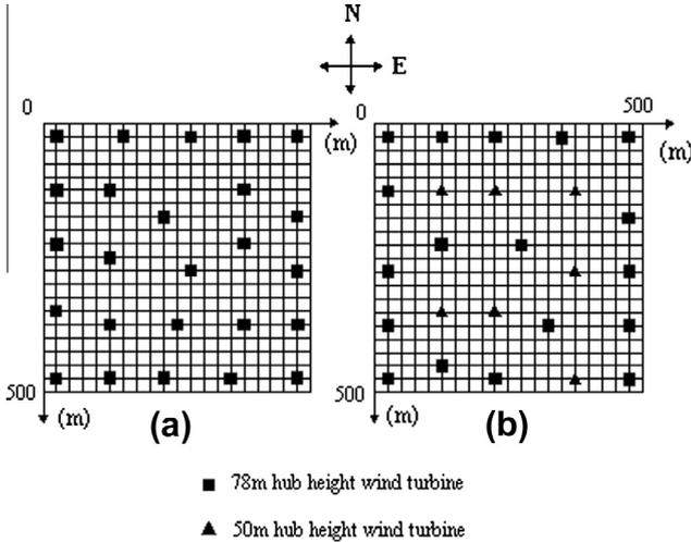
Fig. 6. Optimal layouts generated by GA in second case study: (a) using 78 m hub height wind turbines, (b) using 78 m and 50 m hub heights wind turbines.
