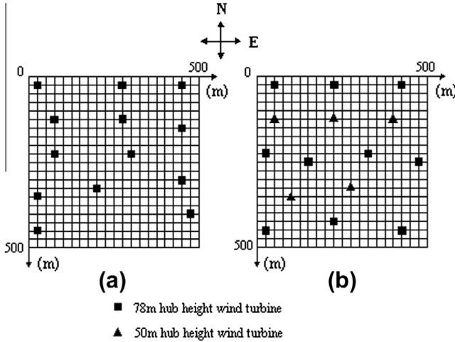
**Fig. 13.** Optimal layouts generated by GA in third case study with comprehensive cost model: (a) using 78 m hub height wind turbines, (b) using 78 m and 50 m hub heights wind turbines.
