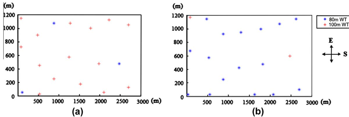
Fig. 15. Typical optimal layouts generated by parallel multi-objective GA optimization with given nameplate capacity: (a) wind farm layout with objective of maximizing power output, (b) wind farm layout with objective of minimizing cost per unit power.
