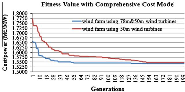
**Fig. 14.** Cost per unit power chart with comprehensive cost model.
