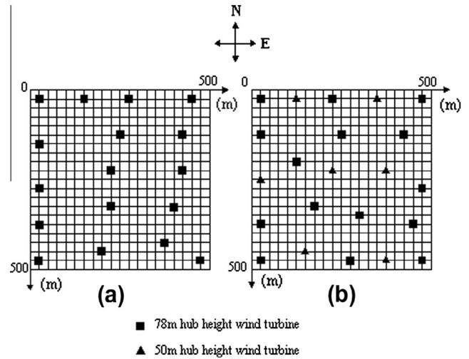
Fig. 11. Optimal layouts generated by GA in third case study with simplified cost model: (a) using 78 m hub height wind turbines, (b) using 78 m and 50 m hub heights wind turbines.
