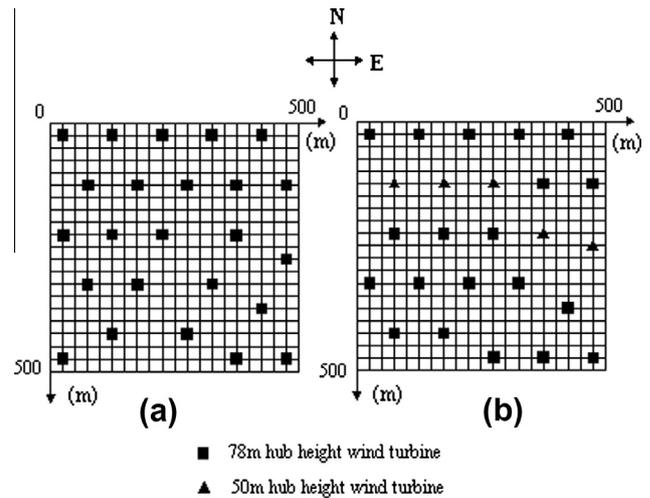
Fig. 4. Optimal layouts generated by GA in first case study: (a) using 78 m hub height wind turbines, (b) using 78 m and 50 m hub heights wind turbines.
