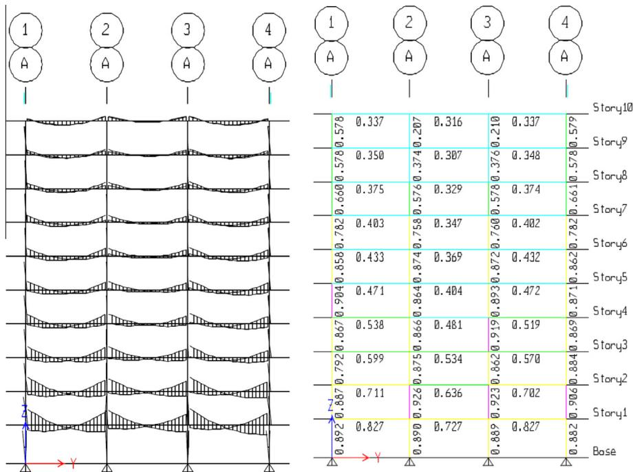
Fig. 4. (a) Bending moment diagram (b) demand/capacity ratio.
