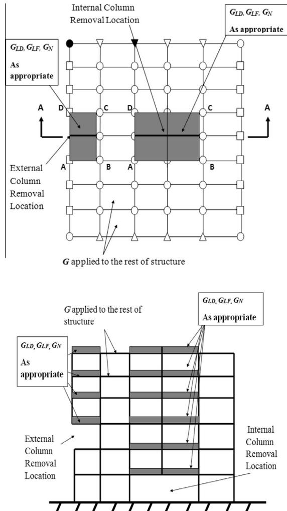
Fig. 2. Gravity load combinations on bays adjacent to the removed column and bays away from the removed column.
