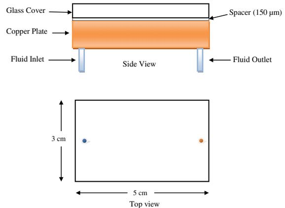
Fig. 4. Experimental schematic of the microsolar thermal collector (Reprinted with permission from Otanicar et al. [28]. Copyright 2010, American Institute of Physics).
