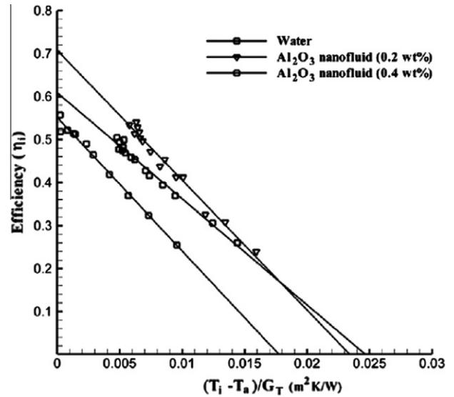
Fig. 12. The efficiencies of solar collectors for Al<sub>2</sub>O<sub>3</sub> nanofluid without surfactant and for water (Reprinted from Yousefi et al. [34], with permission from Elsevier).
