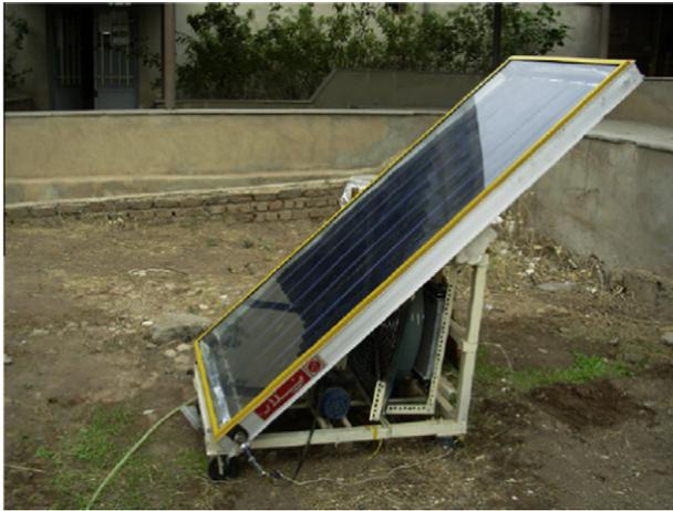
Fig. 10. Flat-plate collector used by Yousefi et al. (Reprinted from Yousefi et al. [34], with permission from Elsevier).
