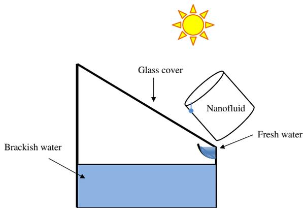
Fig. 15. Schematic of the experimental set up used by Gnanadason et al. [69].
