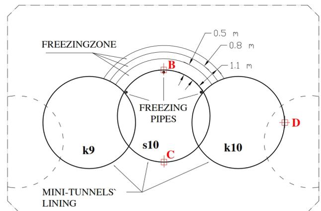
Fig2. Magnified cross section under study.
