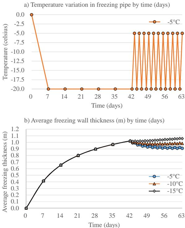
Fig. 5. Creation of frozen wall thickness for different temperature levels  $T_{\max}$ .
