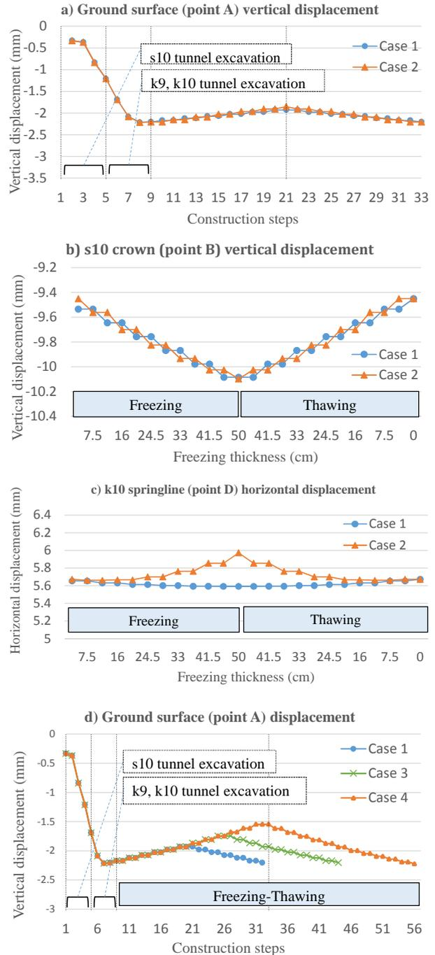
Fig. 3. Freeze-thaw induced displacement (cases of 1, 2, 3 and 4).
