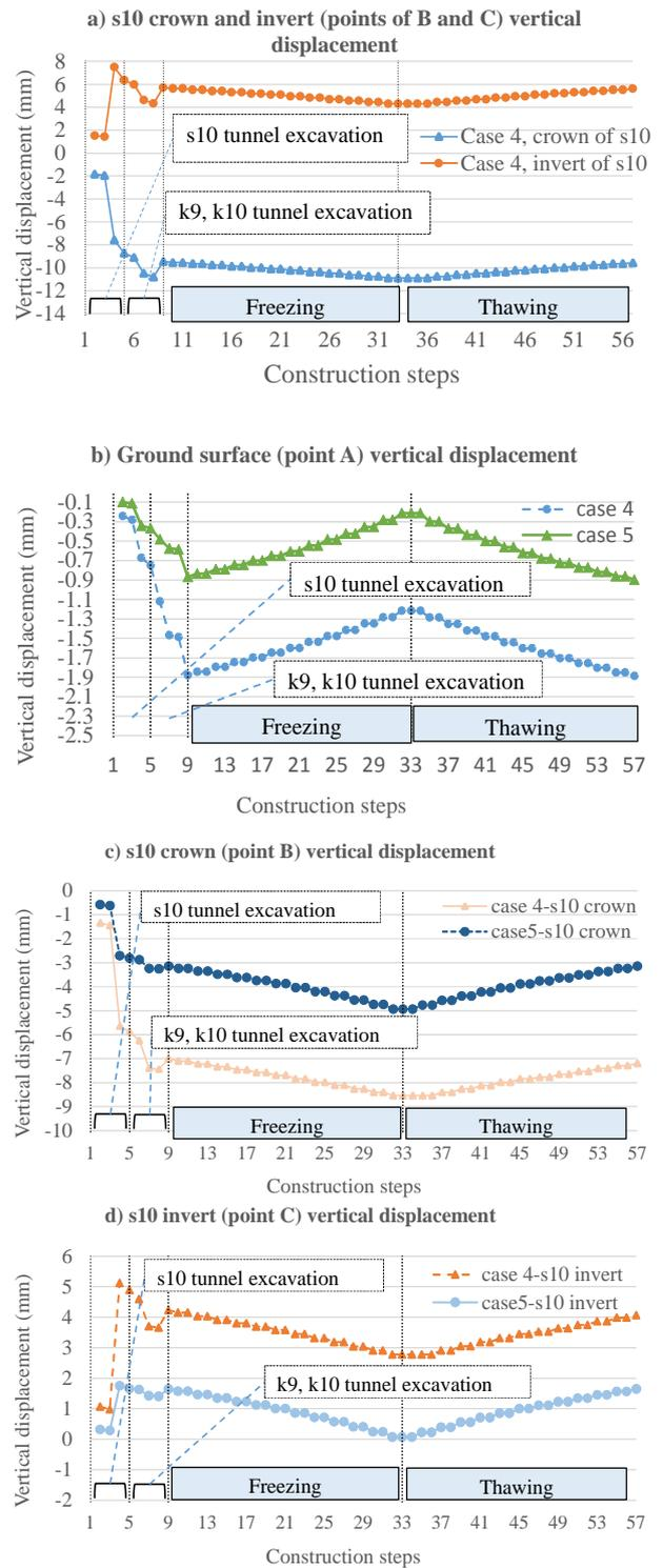
Fig. 4. Freeze-thaw induced displacement (cases of 4 and 5).
