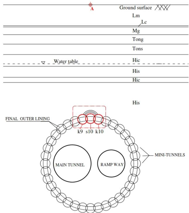
Fig1. Cross section of case study.
