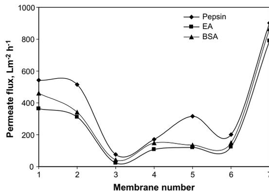
Fig. 3. Permeate flux of various proteins passed through CA membranes with PEG 600.
