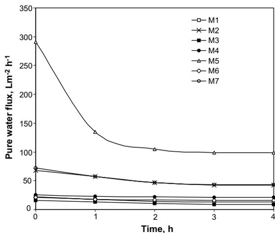
Fig. 1. Effect of time on pure water flux of CA membranes with PEG 600.
