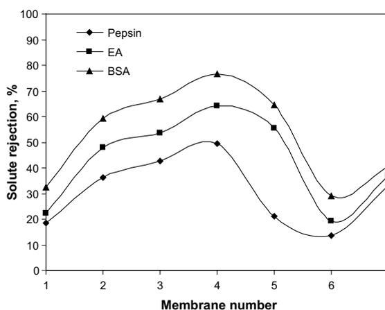
Fig. 4. Percentage rejection of various proteins separated through CA membranes with PEG 600.
