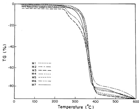
Fig. 5. TGA curves of various CA membranes with PEG 600.
