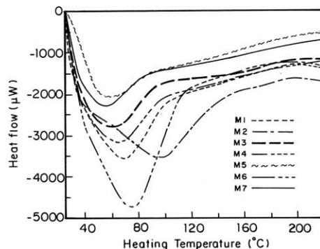
Fig. 6. DSC thermograms of various CA membranes with PEG 600.
