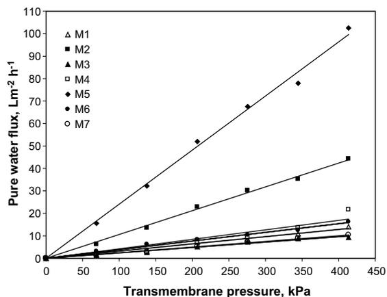
Fig. 2. Effect of transmembrane pressure on pure water flux of CA membranes with PEG 600.
