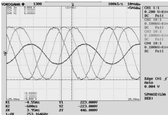
Fig. 9. Output side (five-phase) voltages and current waveform.
