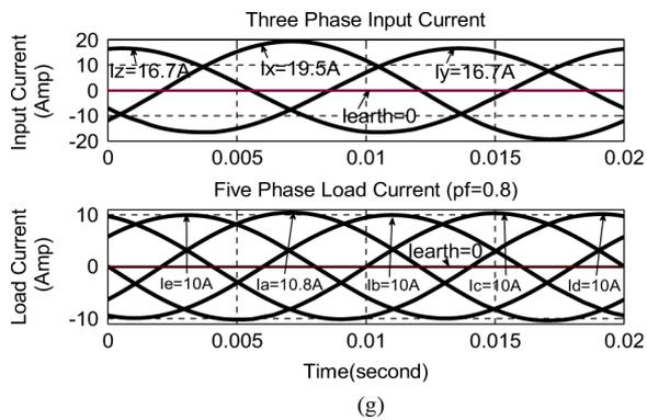
Fig. 5(d)–(g). (d) Input Vz and Vy phases and output Ve phase voltage waveforms. (e) Input three-phase and output five-phase voltage waveforms. (f) Input three-phase and output five-phase load current waveforms at PF = 0.4. (g) Input three-phase and output five-phase load current waveforms at PF = 0.8.
