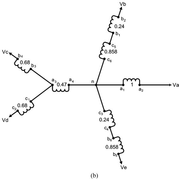
Fig. 2. (a) Proposed transformer winding arrangements (star-star). (b) Proposed transformer winding connection (star).
