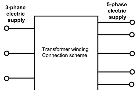
Fig. 1. Block representation of the proposed system.
